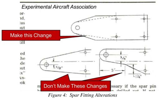
The corrected fittings, on the lower part of this figure, should only be made if you did NOT correct the fuselage dimensions in Companion Guide #3.
