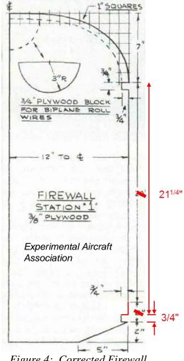
Figure 4: Corrected Firewall
