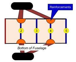
Figure 15: Landing Gear Reinforcement Locations
