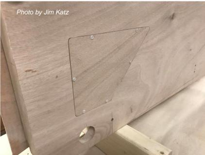
Figure 38: Aft Fuselage Inspection Cover (Fuselage is Upside-Down)
