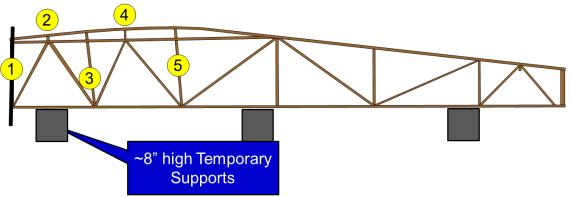
Figure 5: Fuselage Positioned for Station 2 Installation
