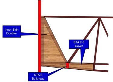
Figure 12: Forward Inner Reinforcement
