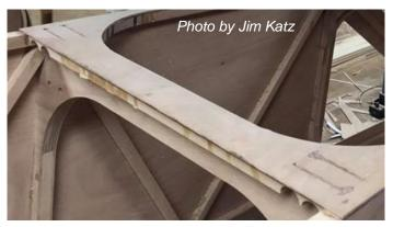
Figure 25: Slots for Landing Wire Anchors
