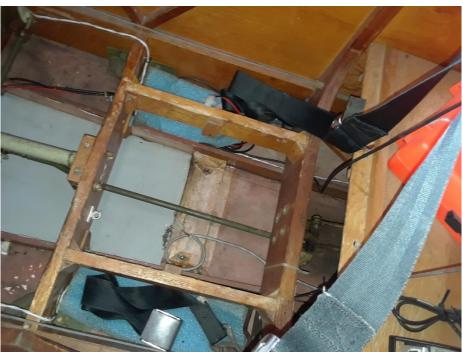
Figure 14: Seat Support Rails
