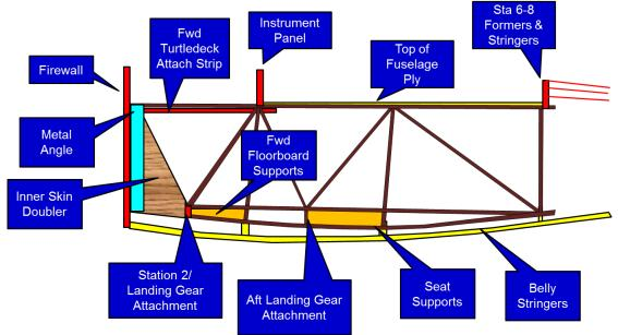
Figure 1: Secondary Fuselage Structure
