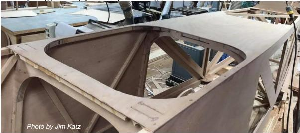
Figure 24: Cockpit-Area Plywood
