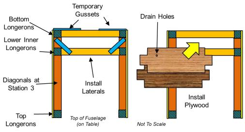
Figure 11: Station 2 Construction
