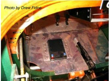
Figure 42: Drew Fidoe's Battery Installation
