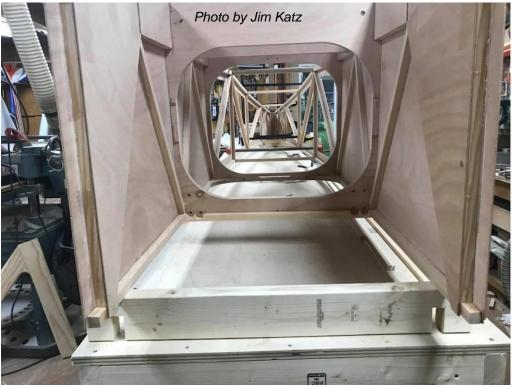
Figure 13: Photo of Inner Skin Reinforcement
