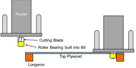
Figure 26: Using a Flush Trim Bit
