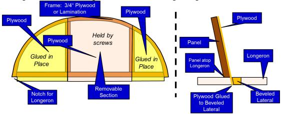
Figure 27: Instrument Panel
