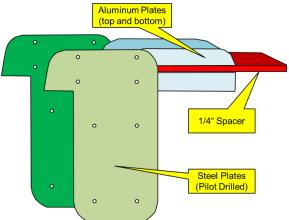
Figure 18: Landing Wire Anchors
