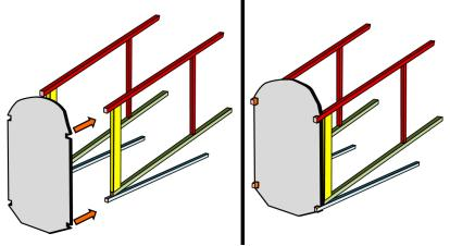
Figure 7: Firewall Fitting
