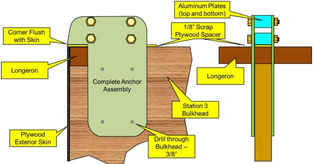
Figure 20: Landing Wire Anchor Installation
