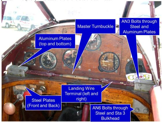
Figure 19: Landing Wire Support Assemblies
