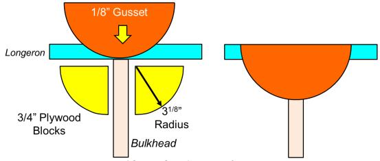
Figure 16: Landing Gear Reinforcements
