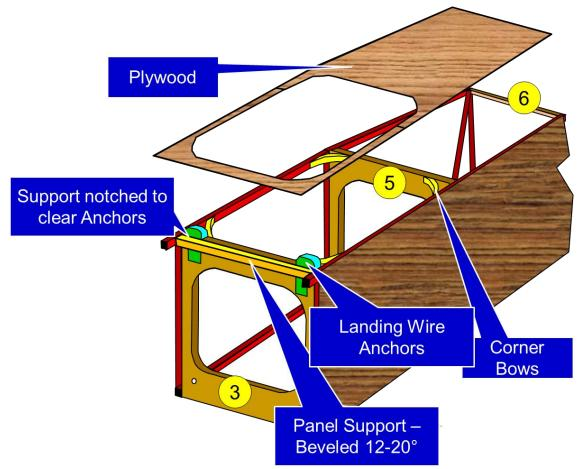
Figure 21: Cockpit Top Plywood
