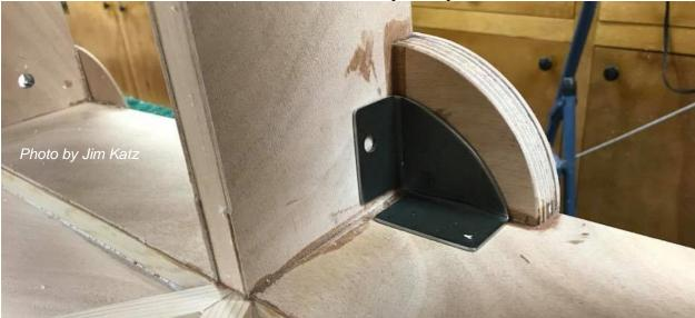
Figure 17: Landing Gear Reinforcement with Bracket
