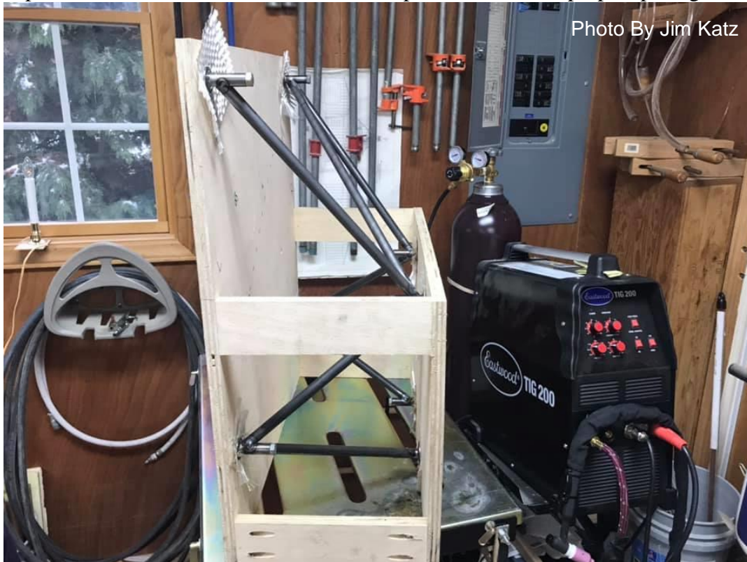
Figure 28: Jig for Welding Engine Mount
