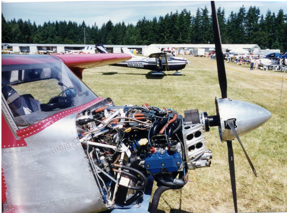
Figure 8: Subaru Engine Installed on Murphy Rebel
