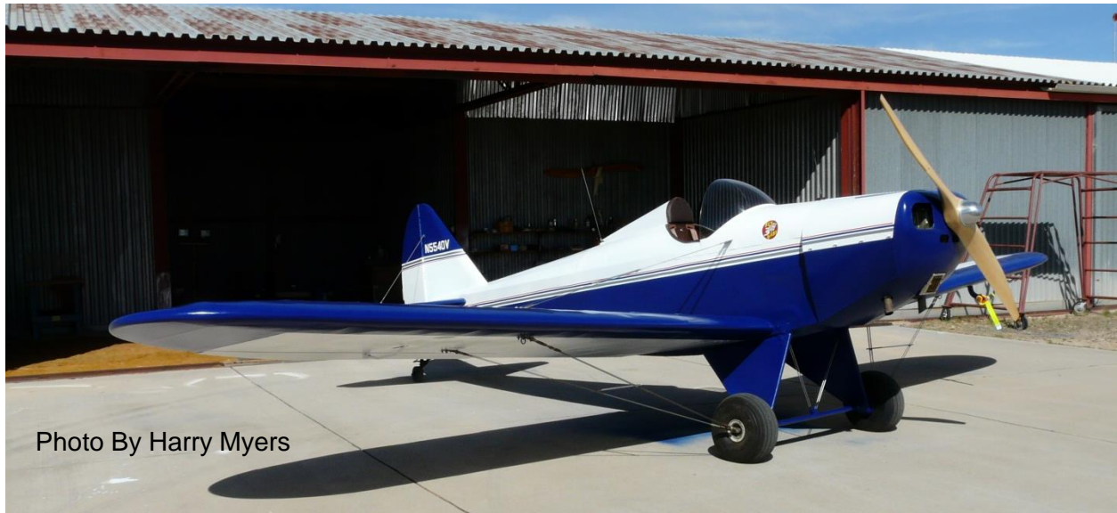
Figure 33: Fly Baby with Pressure Cowling
