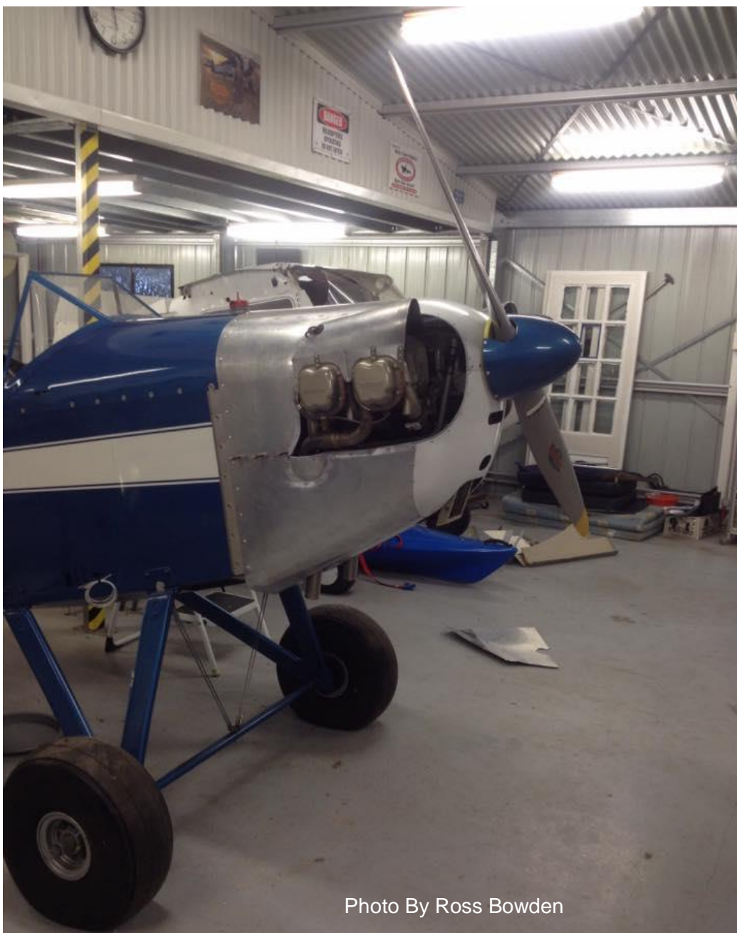
Figure 45: Cowling Without Forward Attachment
