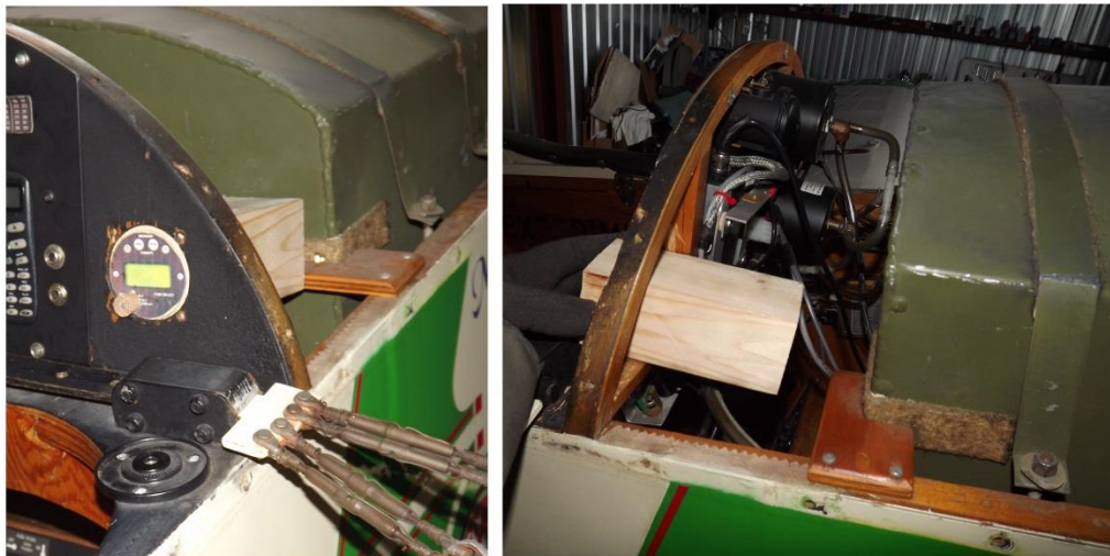
Figure 54: Wooden Mockup of Transponder for Fit Check
