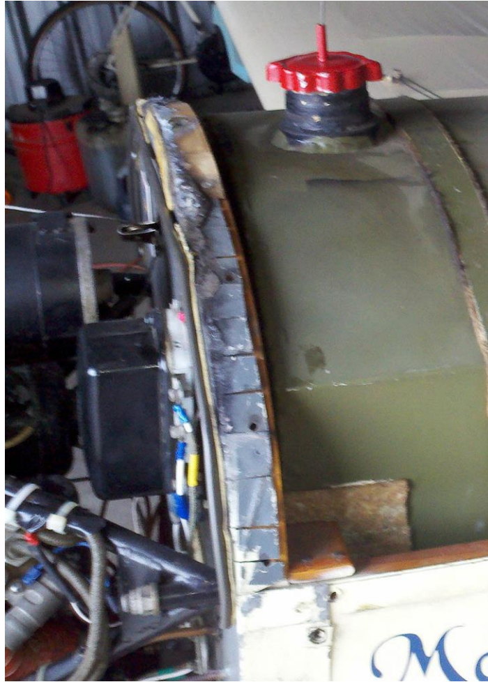
Figure 24: Slitted/Bent Firewall Metal
