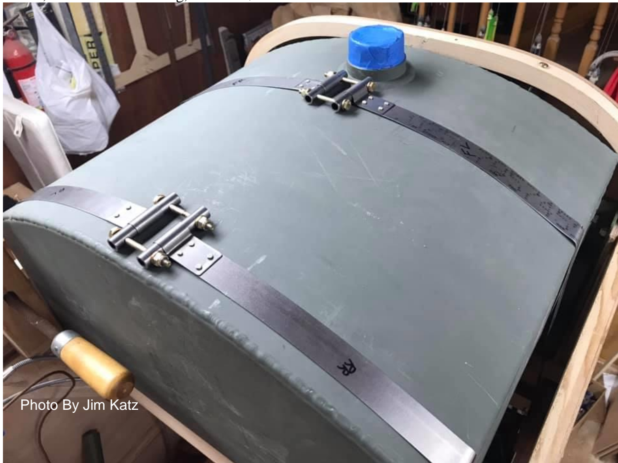
Figure 55: Aircraft Spruce and Specialty Fly Baby Fuel Tank
