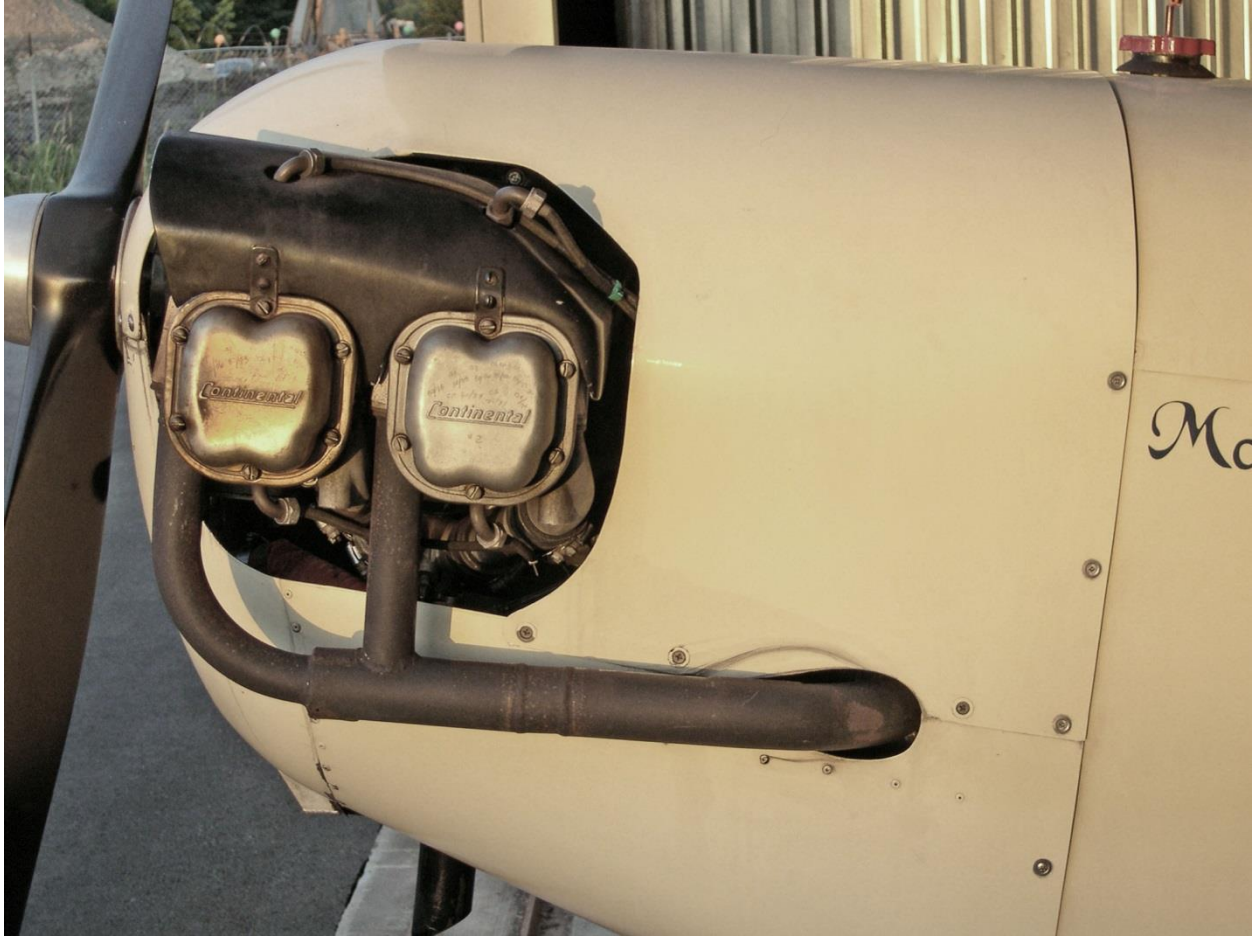
Figure 42: Hole in Cowling for Exhaust Pipe
