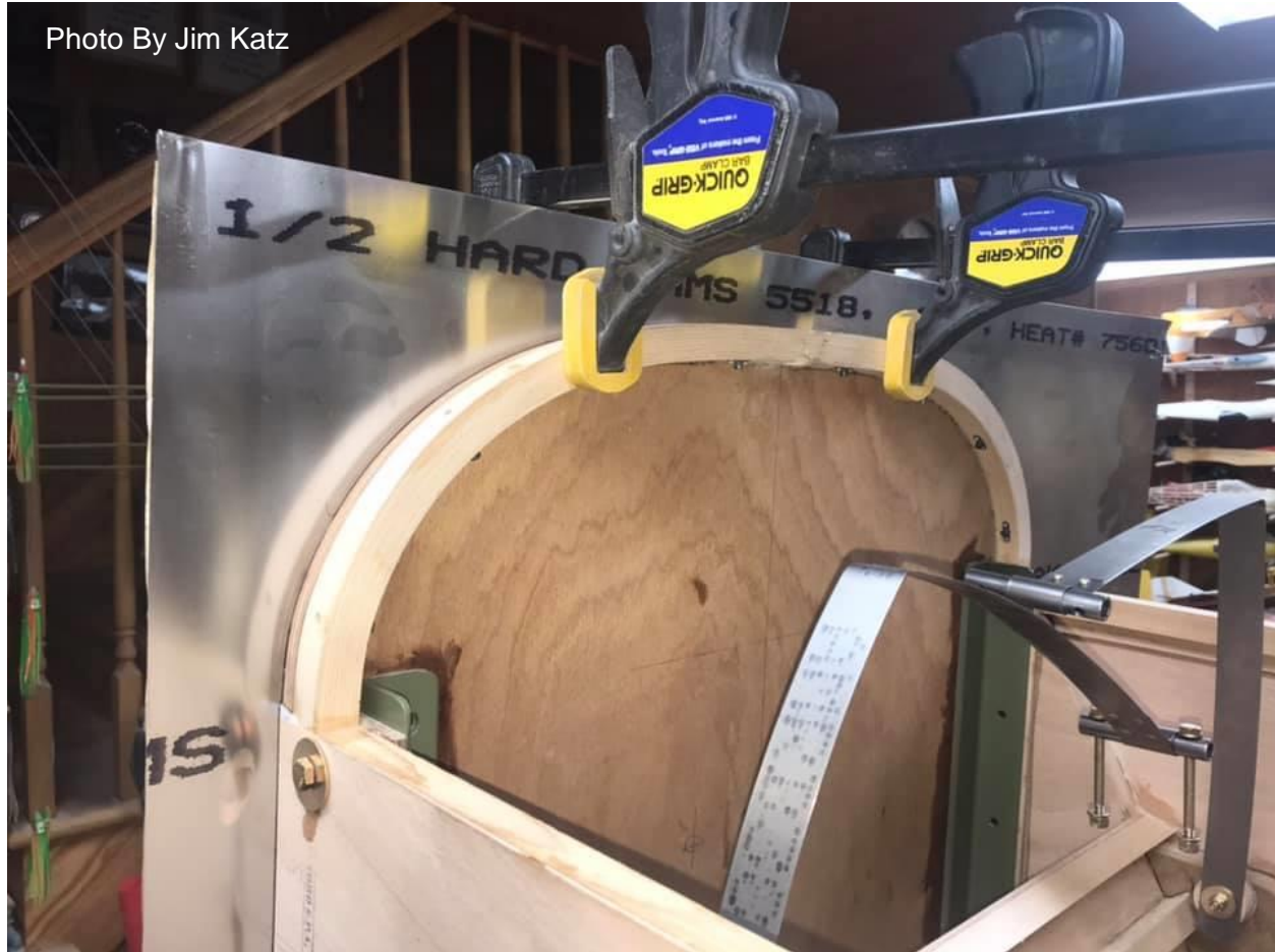
Figure 25: Matching the Bulkhead Shape for the Firewall
