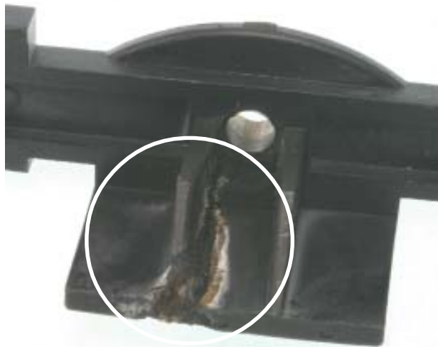
Unacceptable (Developing bearing bar failure)
