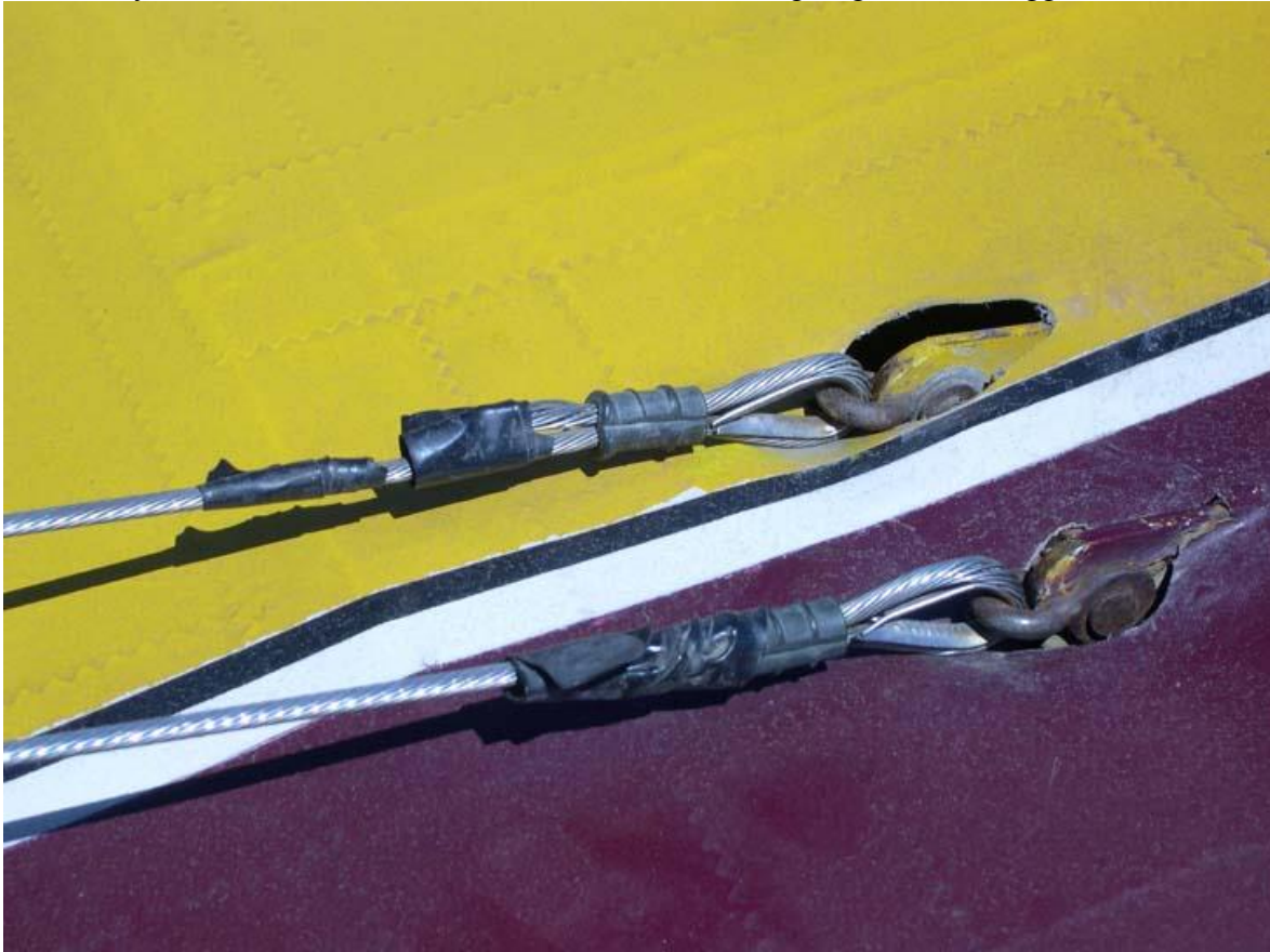
Figure 16: N500F Wire Attachment, without Tab
