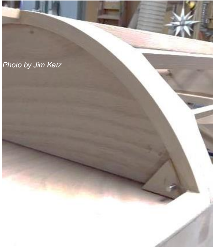
Figure 19: Aft Corner Reinforcement on the Turtledeck
