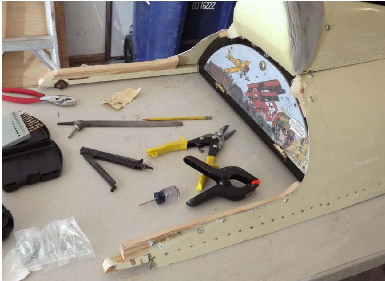
Figure 29: Reinforcement for Ingress/Egress on Modified Coaming
