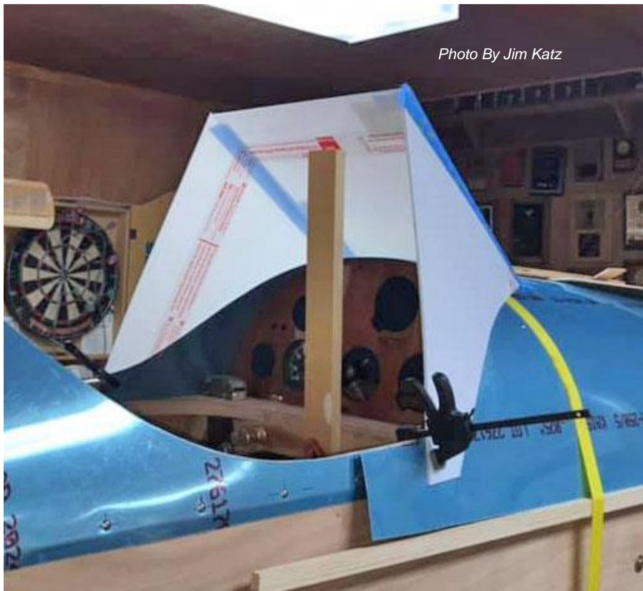
Figure 7: Windshield Panels Temporarily in Place
