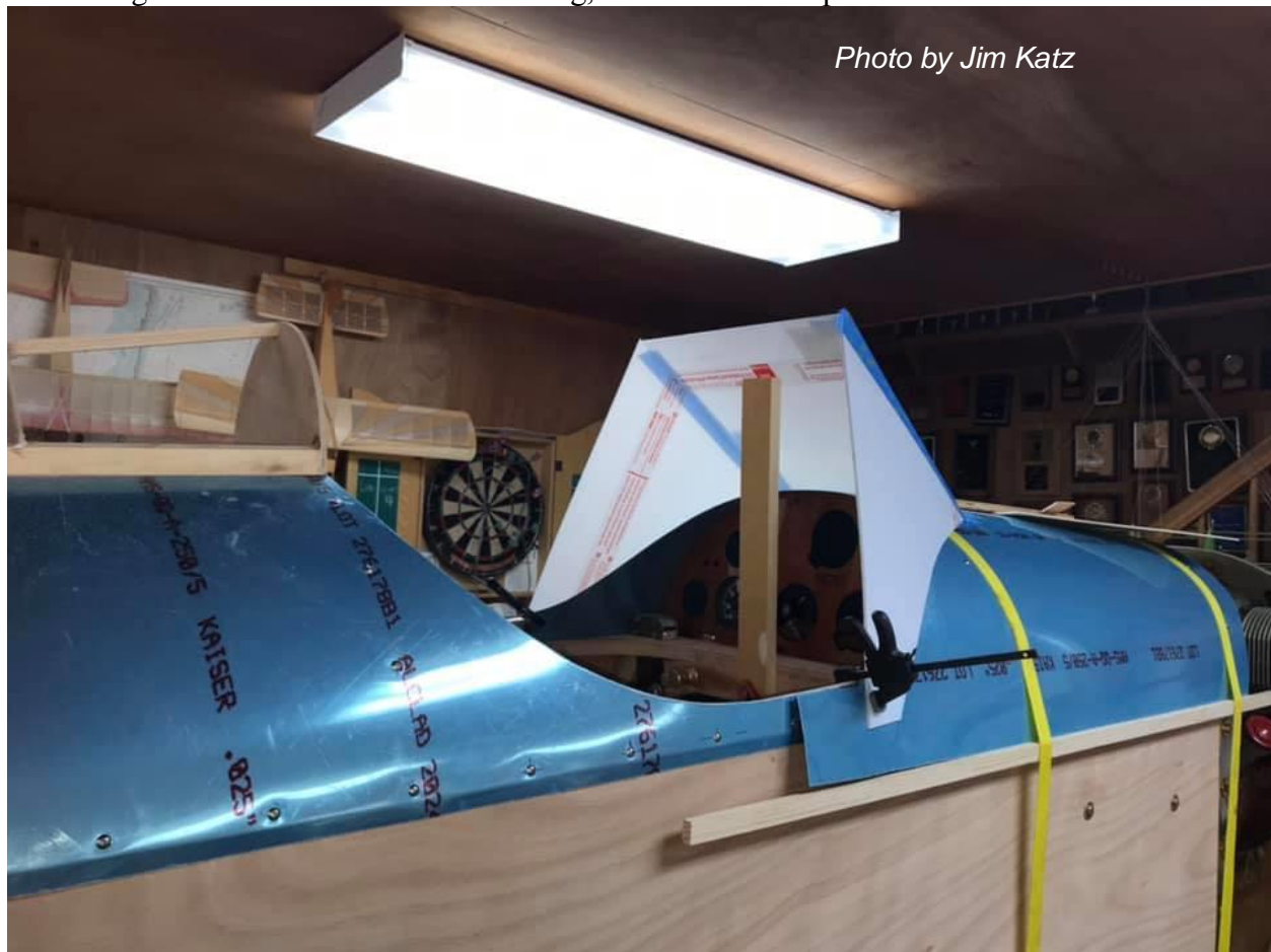
Figure 23: Coaming Cut to Fit
