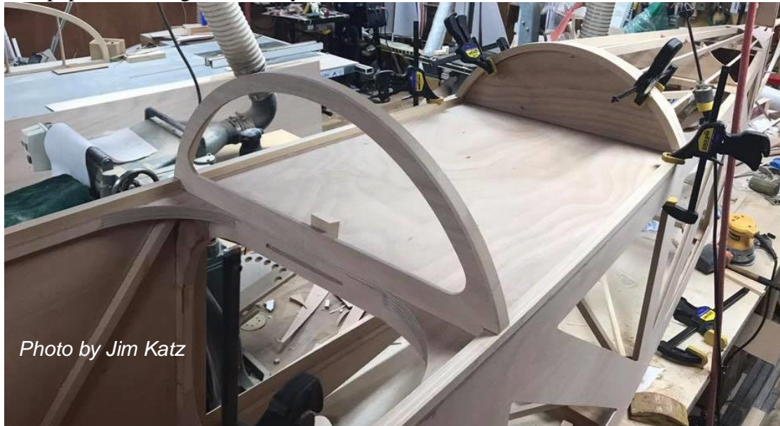
Figure 21: Turtleneck Frame in Progress
