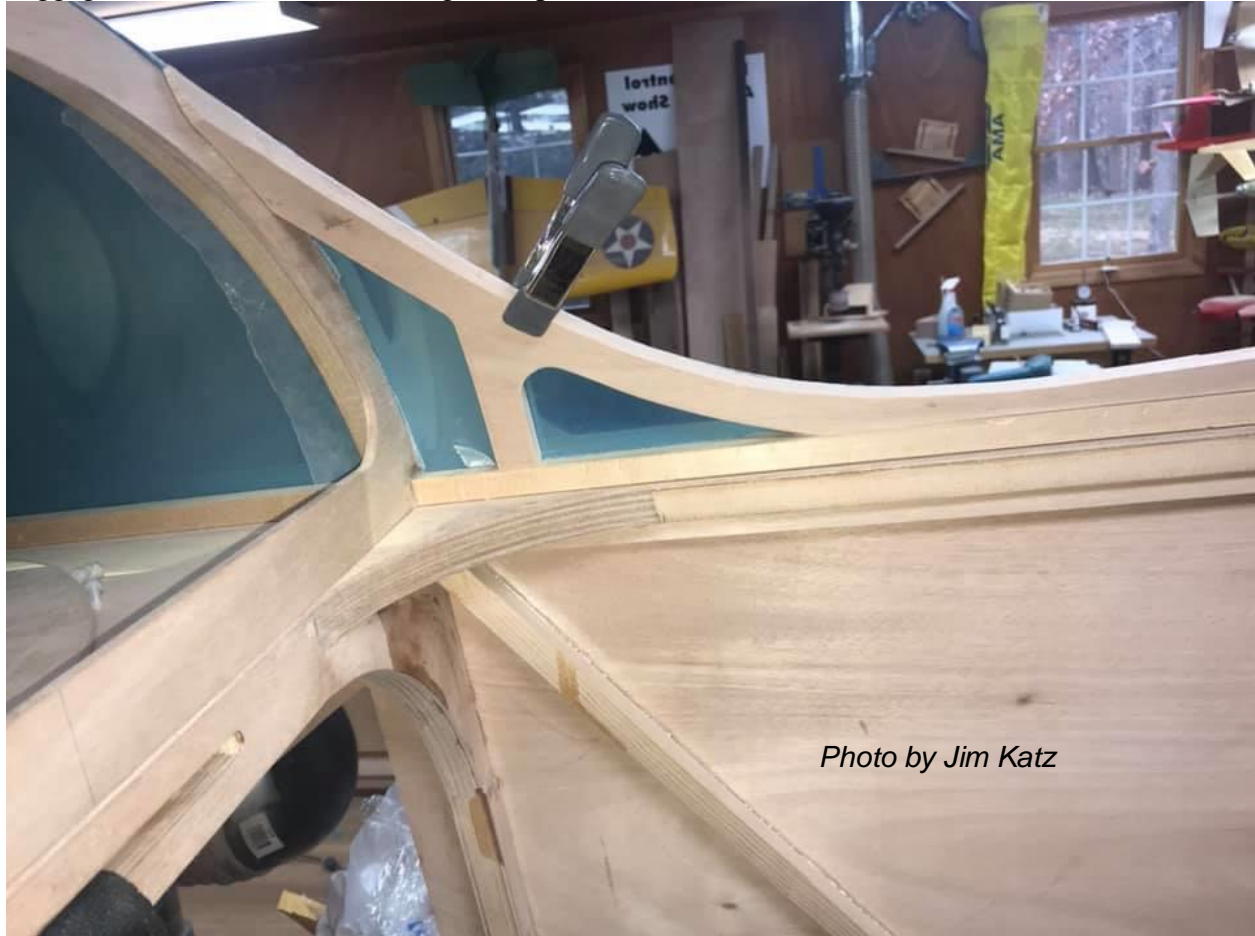
Figure 28: Coaming Reinforcement In Place
