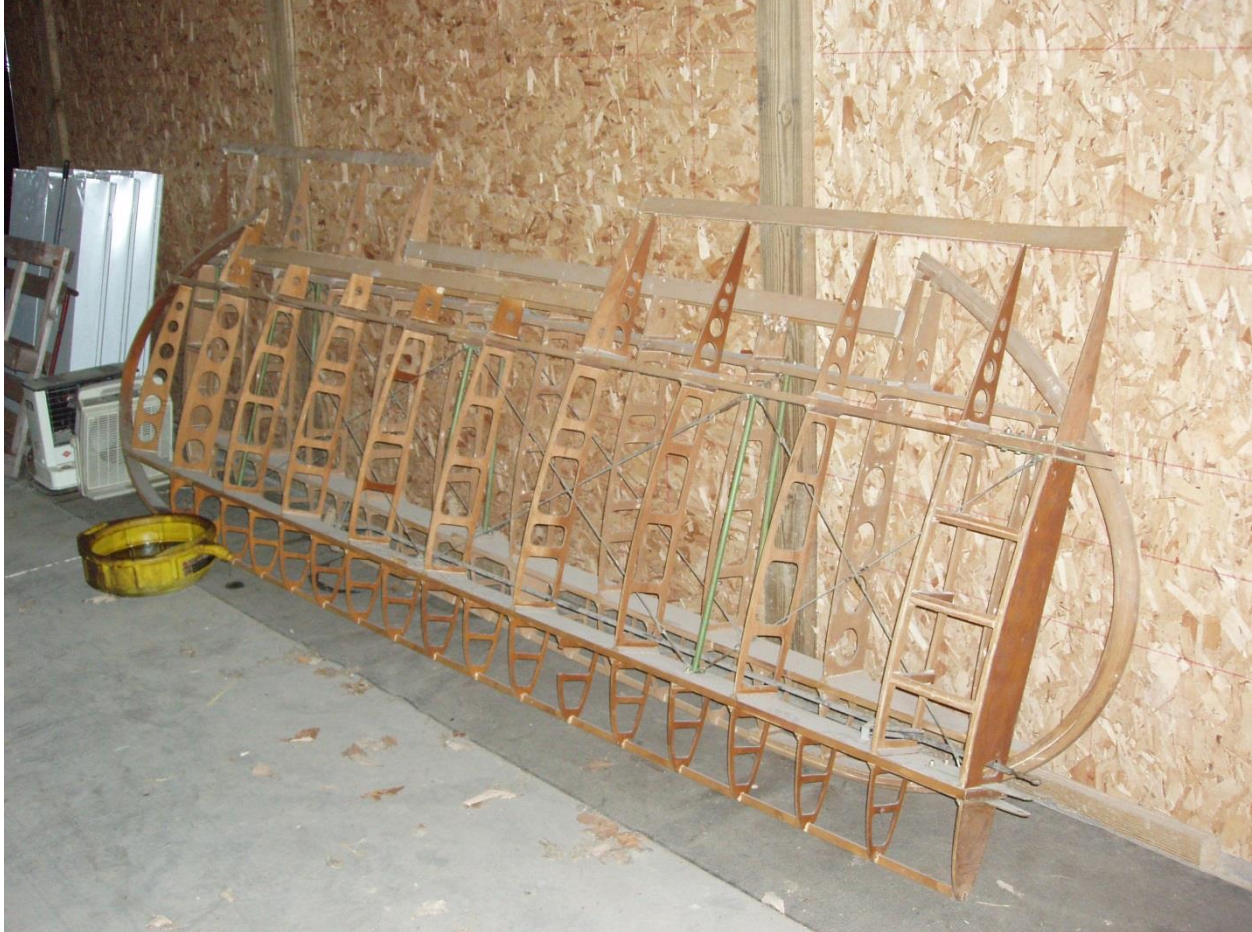
Figure 62: Wing Ribs with Lightening Holes
