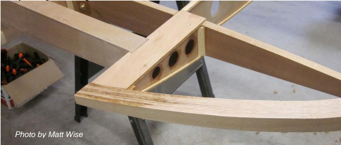
Figure 43: Trailing Edge Close-Up
