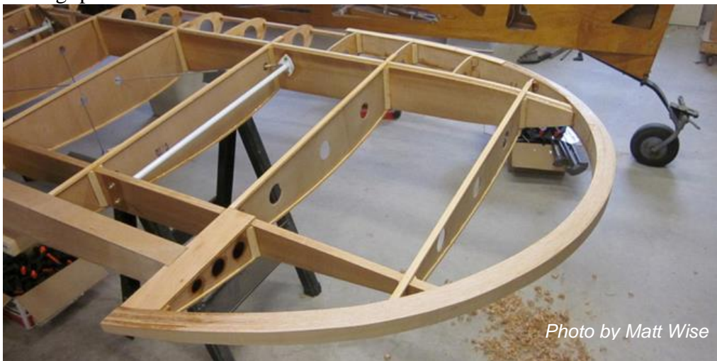
Figure 40: All Laminations Applied
