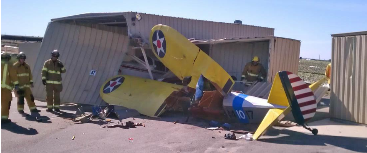
Figure 45: Wingtips Intact After Hangar Crash
