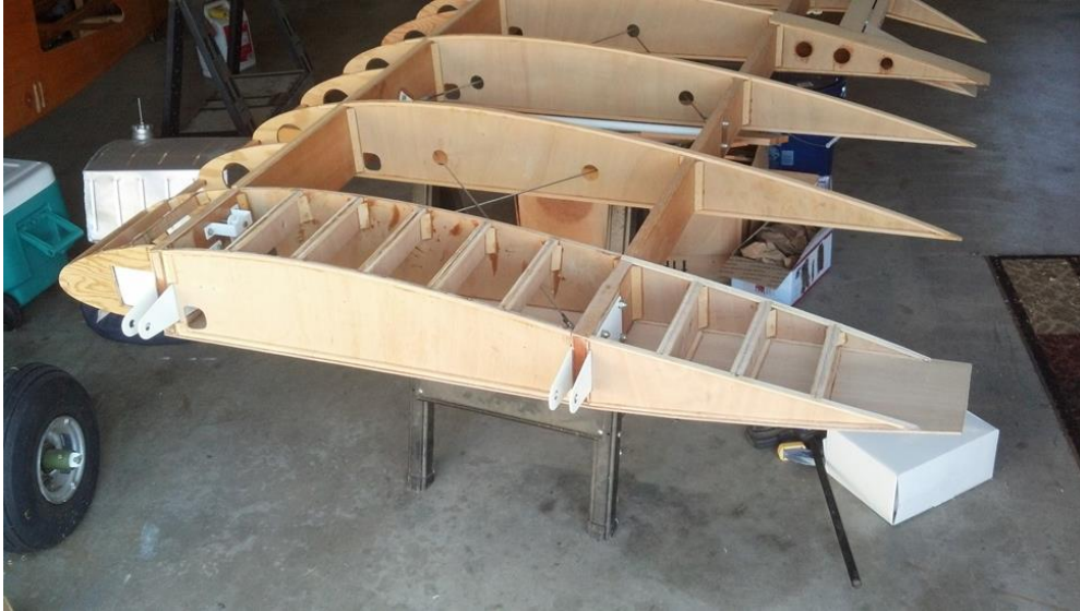
Figure 58: Wing Walk Support Intercostals
