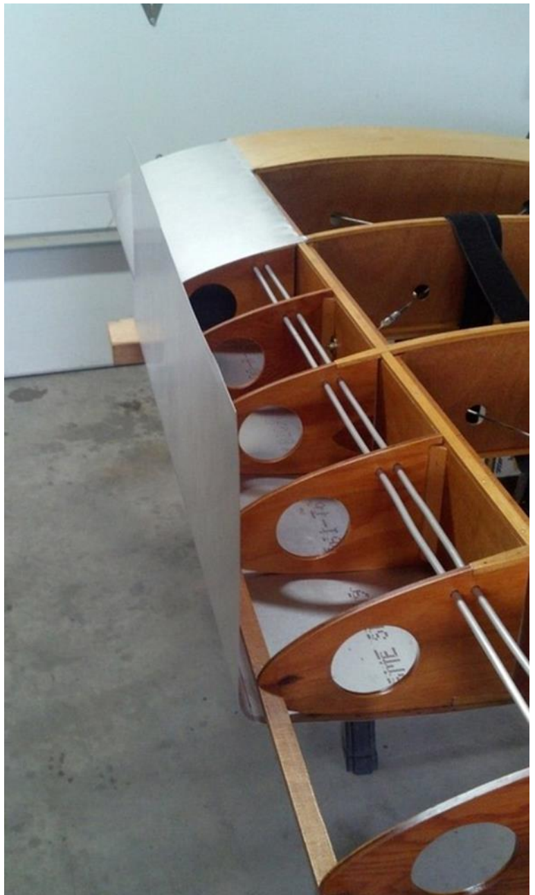
Figure 59: Covering Leading Edge
