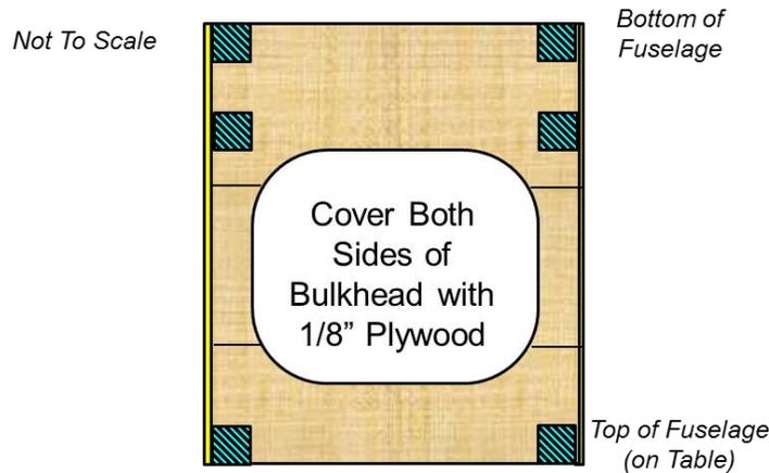
Figure 37: Completing the Bulkhead
