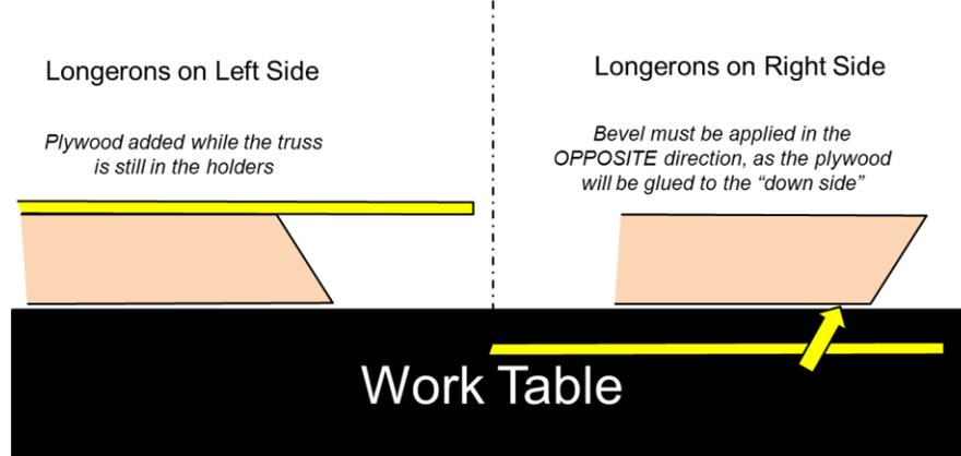
Figure 61: Applying the Tail Beveling During Assembly Has to be Done Carefully
