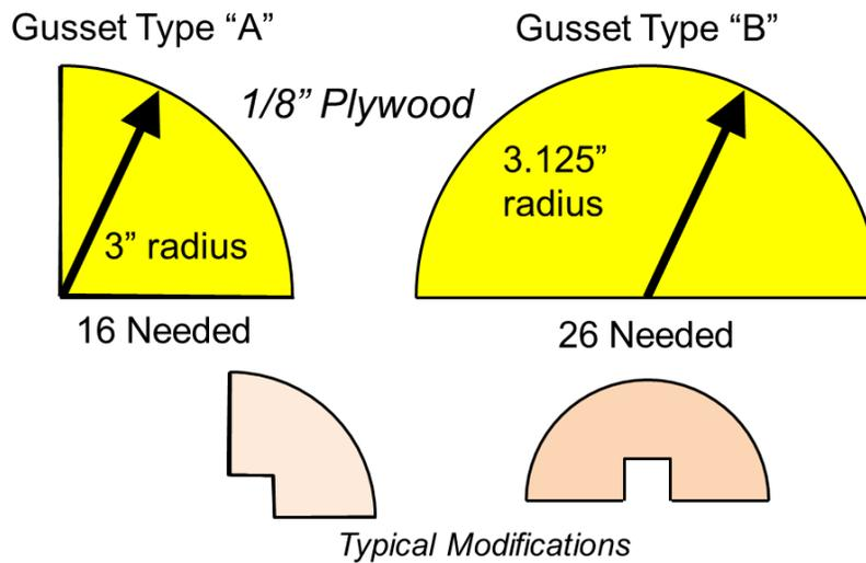
Figure 46: Gussets for Fuselage Assembly
