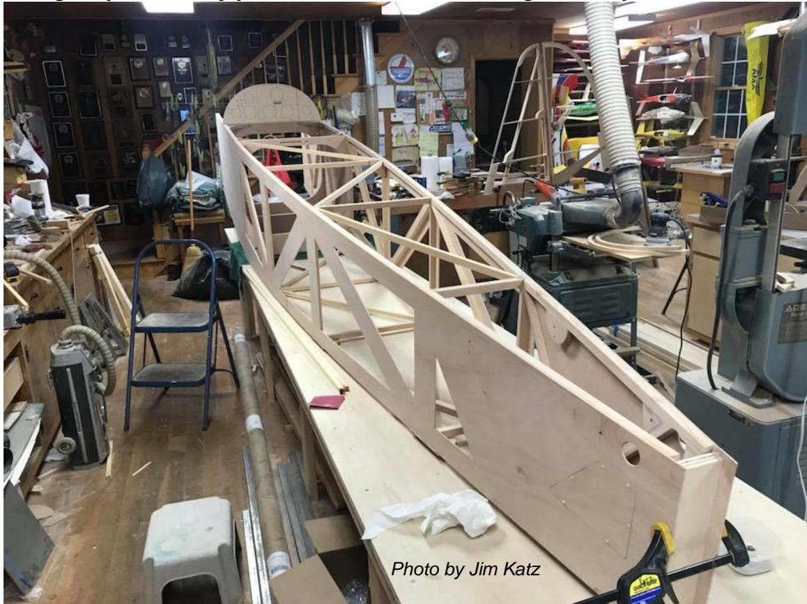
*Figure 71: Routed Fuselage*
