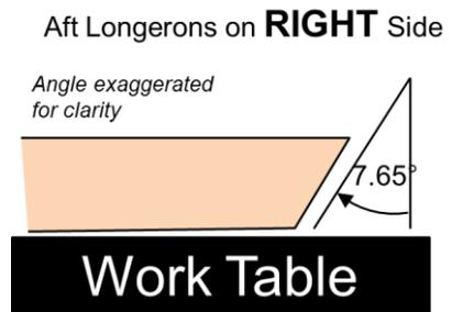
Figure 25: Aft Longeron Beveling on Right Side of Fuselage
