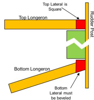
Figure 65: Bevel in Lower Lateral
