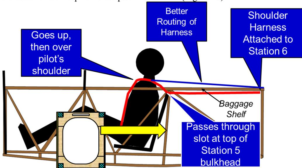
Figure 72: Shoulder Harness Routing
