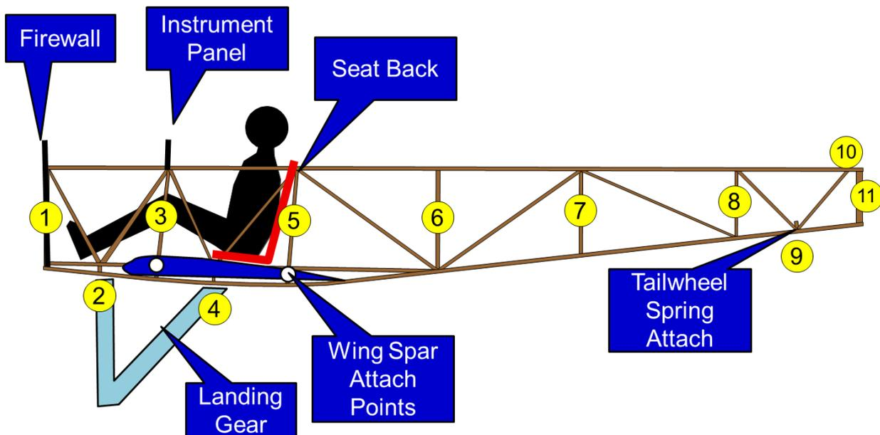
Figure 3: Fuselage Stations
