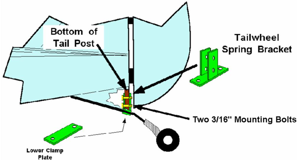
Figure 54: Tailwheel Spring Support Bracket
