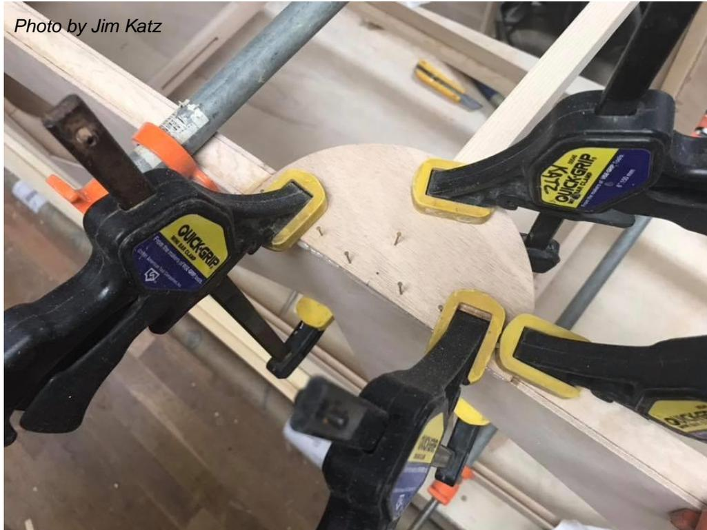
Figure 47: Gluing the Gussets
