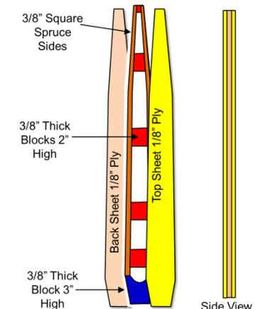
Figure 51: Stock Rudder Post Construction
