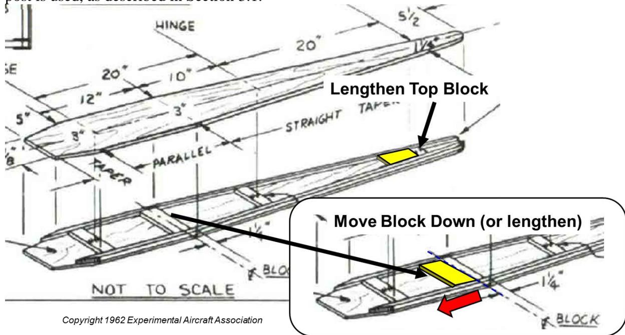
Figure 7: Rudder Post Block Correction
