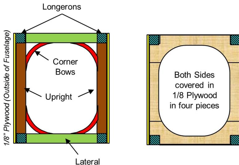
Figure 29: Bulkhead Construction
