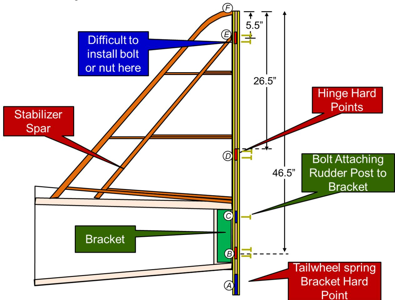
*Figure 53: Interference Issue with Upper Hinge Point*
