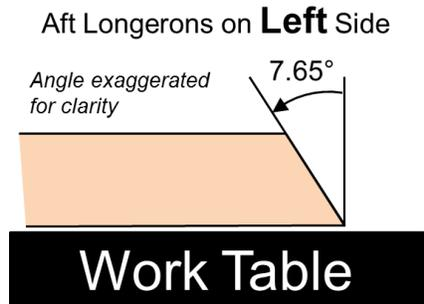
Figure 13: Aft Longeron Bevel on LEFT side of Fuselage
