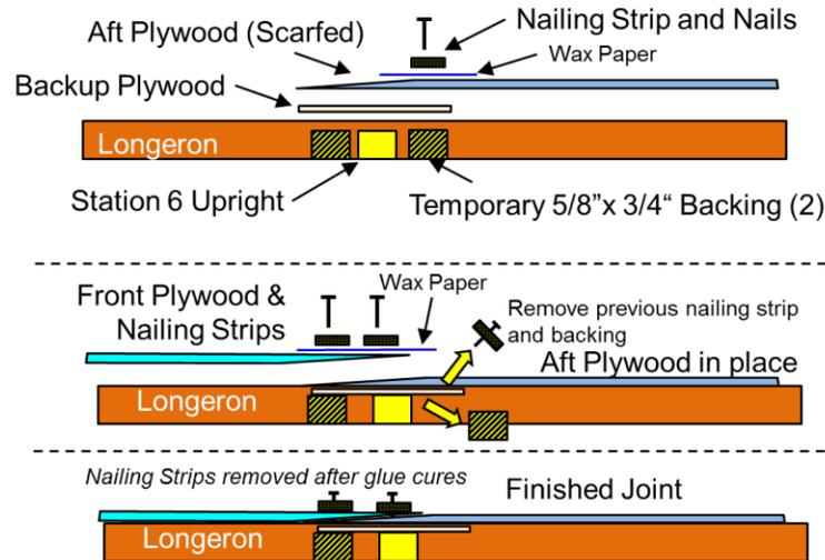
Figure 22: Cross-Sectional View of Station 6 Plywood Scarf
