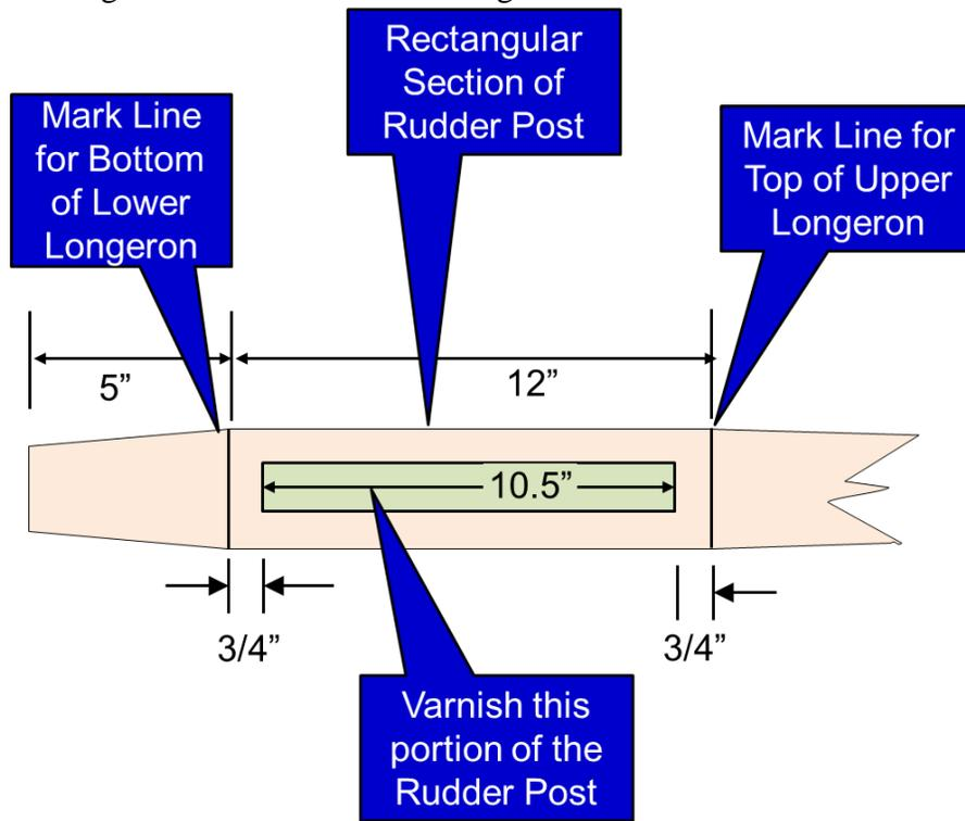
Figure 58: Rudder Post Preparation
