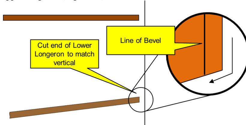
Figure 12: Trimming Back End of Lower Longeron
