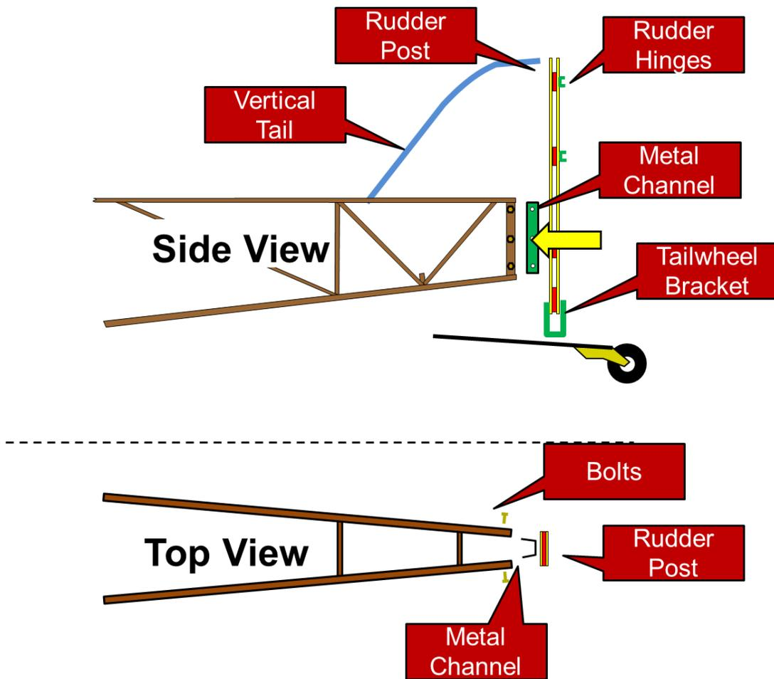
Figure 50: Rear Fuselage Joining
