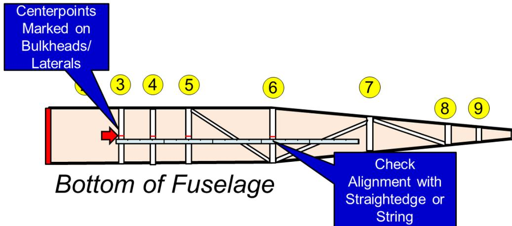
Figure 48: Suggested Alignment Check
