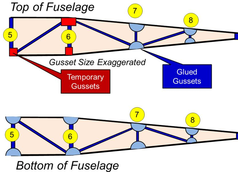
Figure 49: Gusseting the Aft Fuselage
