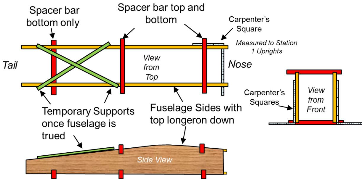
Figure 32: Aligning the Fuselage Sides
