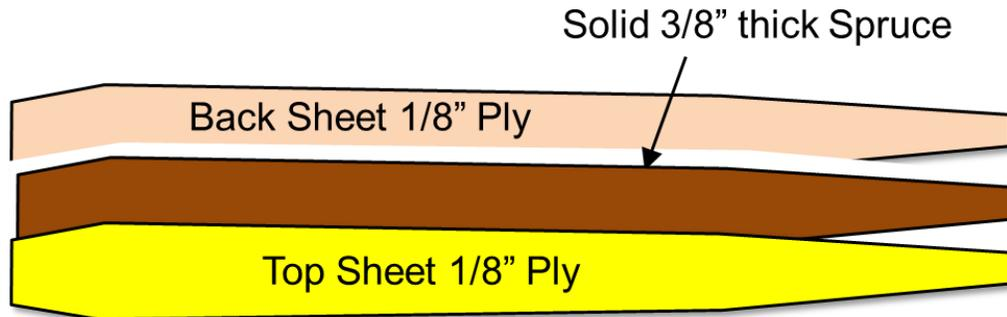
*Figure 56: Solid-Core Rudder Post*
