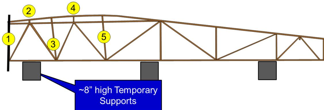
Figure 5: Fuselage Positioned for Station 2 Installation
