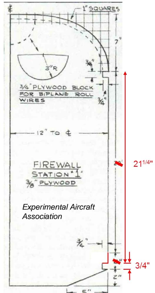
Figure 4: Corrected Firewall
