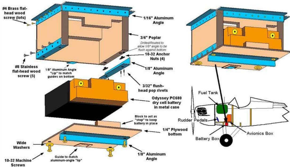
Figure 43: Battery Holder for Odyssey PC680 Battery
