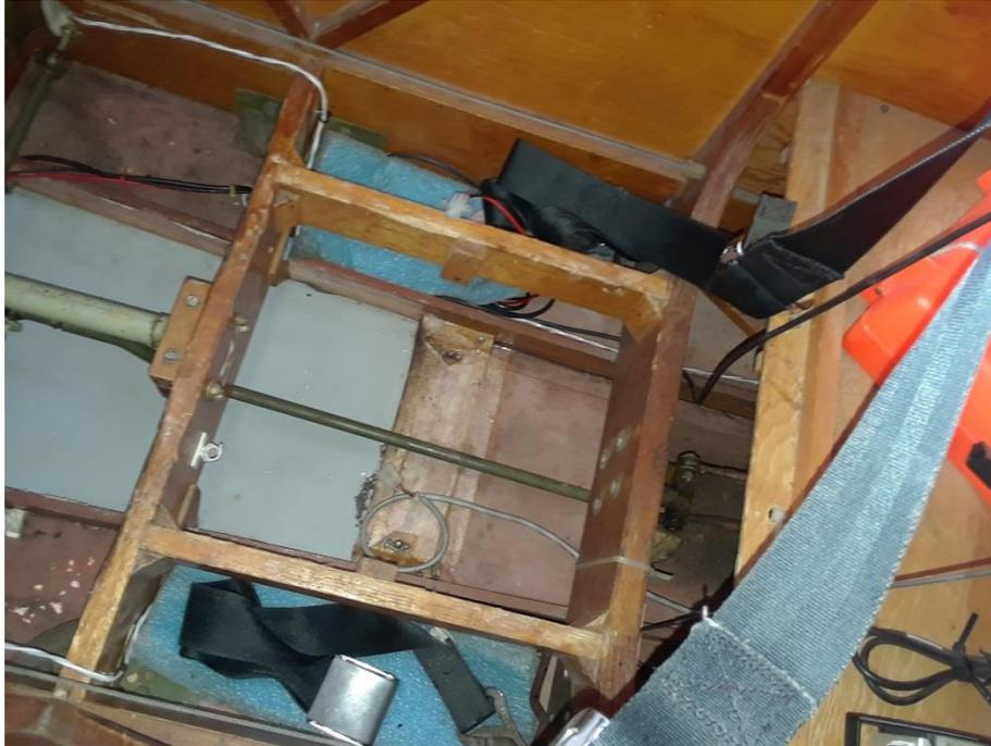
Figure 14: Seat Support Rails
