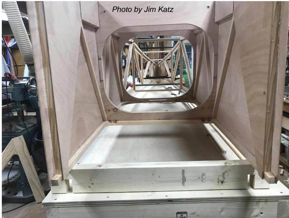
*Figure 13: Photo of Inner Skin Reinforcement*
