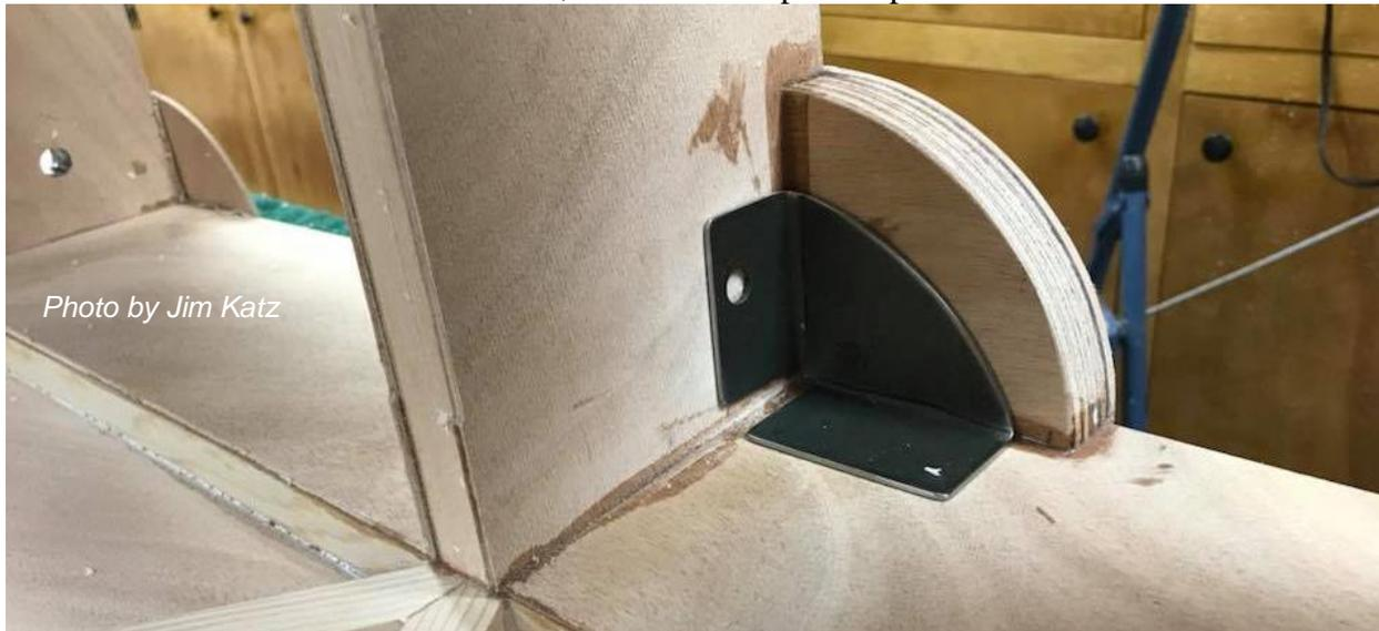
Figure 17: Landing Gear Reinforcement with Bracket
