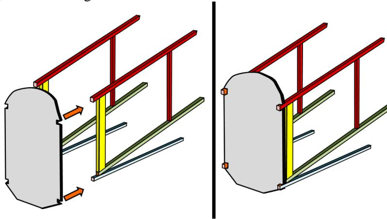
*Figure 7: Firewall Fitting*
