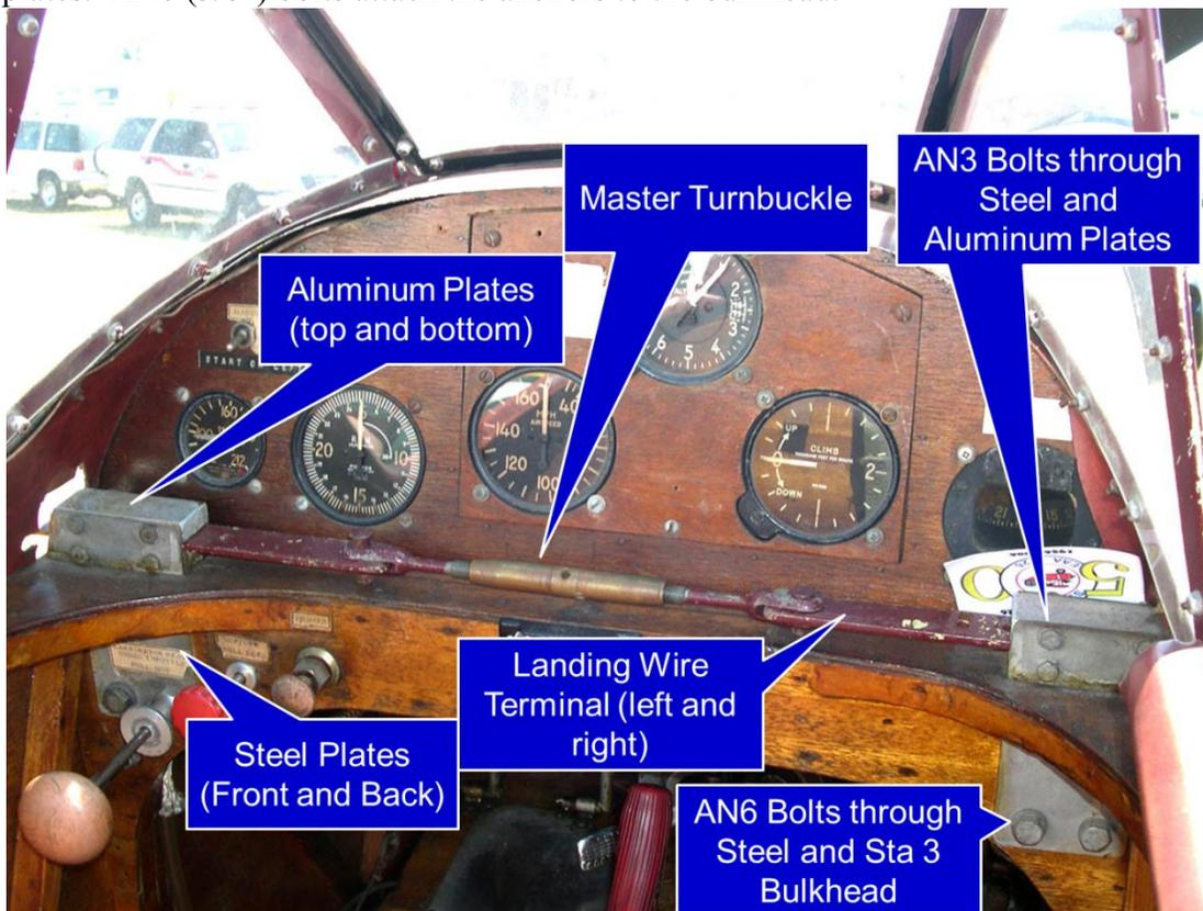
Figure 19: Landing Wire Support Assemblies
