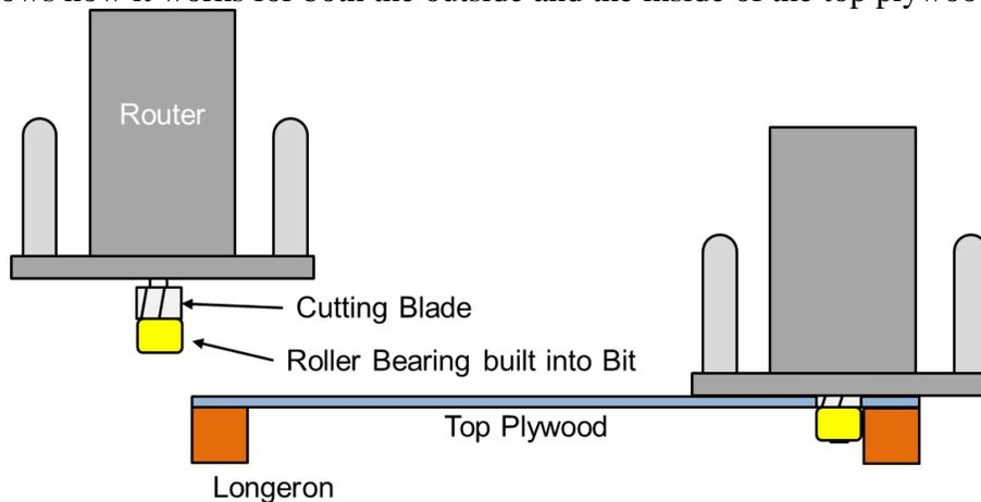
Figure 26: Using a Flush Trim Bit
