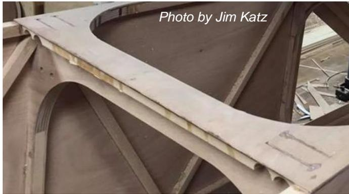
Figure 25: Slots for Landing Wire Anchors
