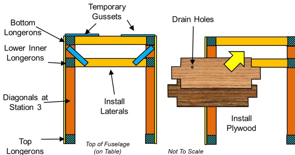
Figure 11: Station 2 Construction
