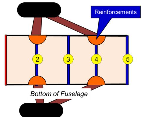
Figure 15: Landing Gear Reinforcement Locations
