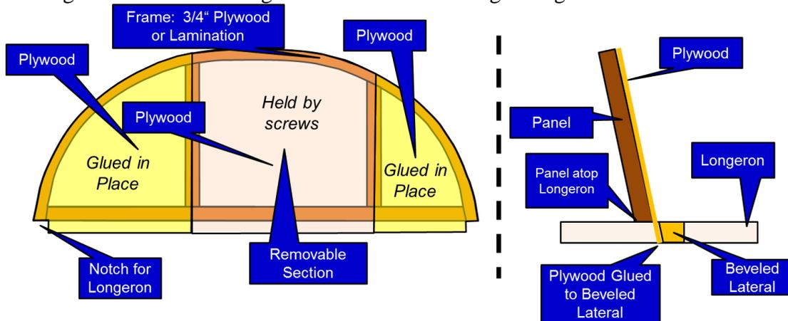
Figure 27: Instrument Panel
