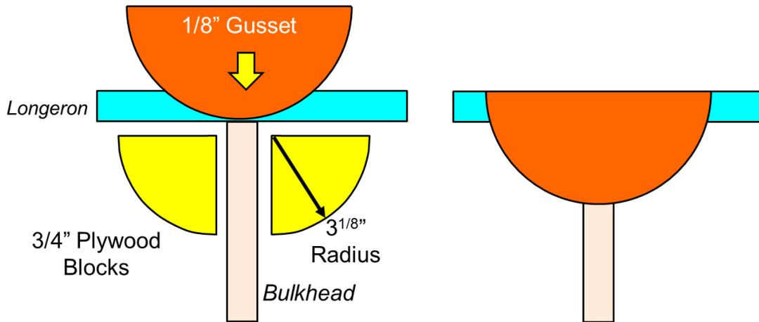
Figure 16: Landing Gear Reinforcements
