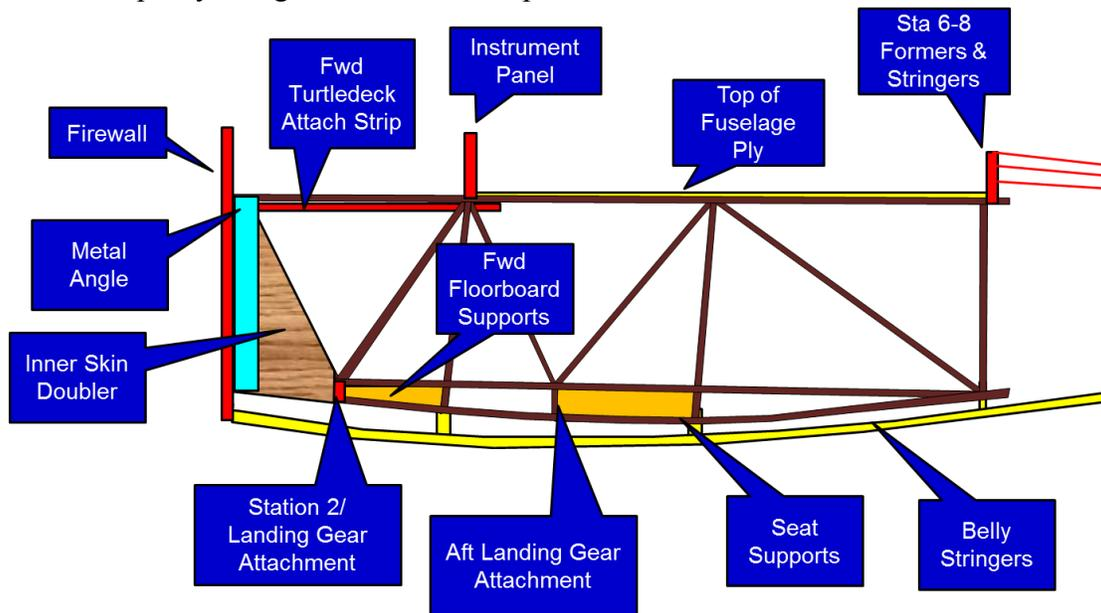
Figure 1: Secondary Fuselage Structure
