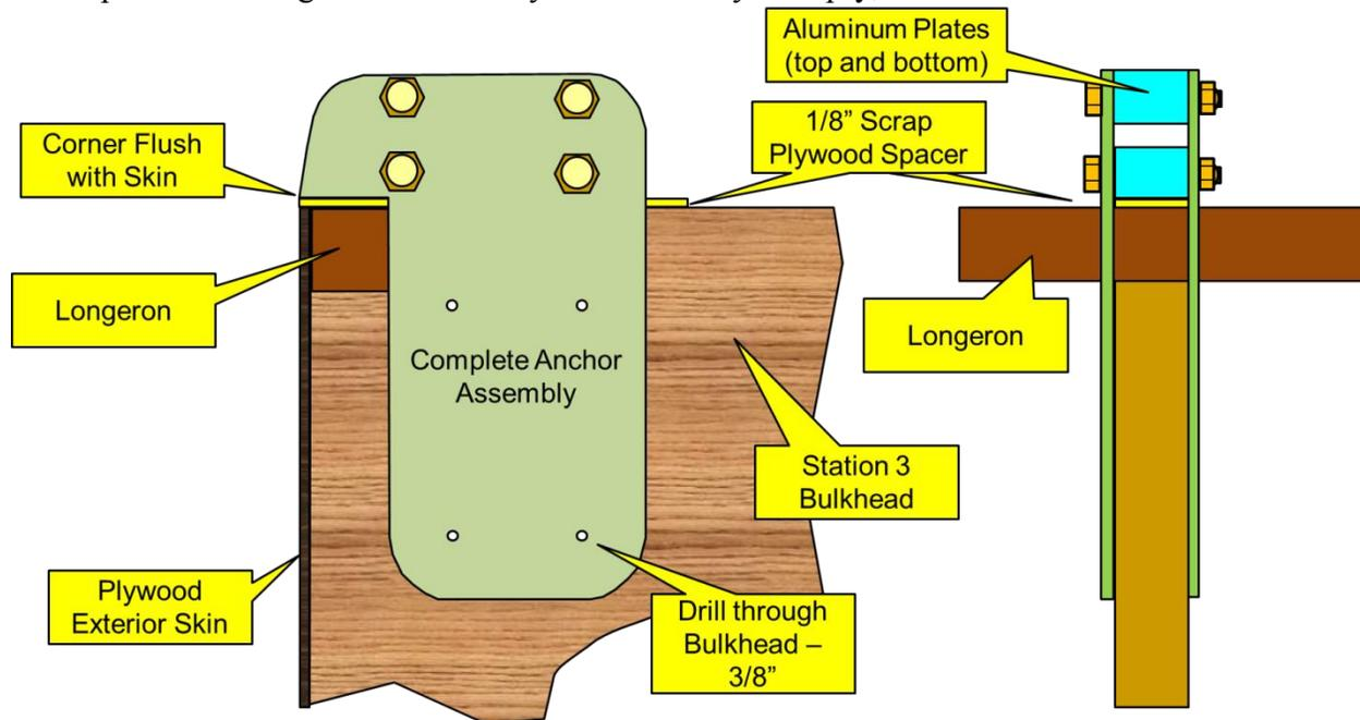
Figure 20: Landing Wire Anchor Installation
