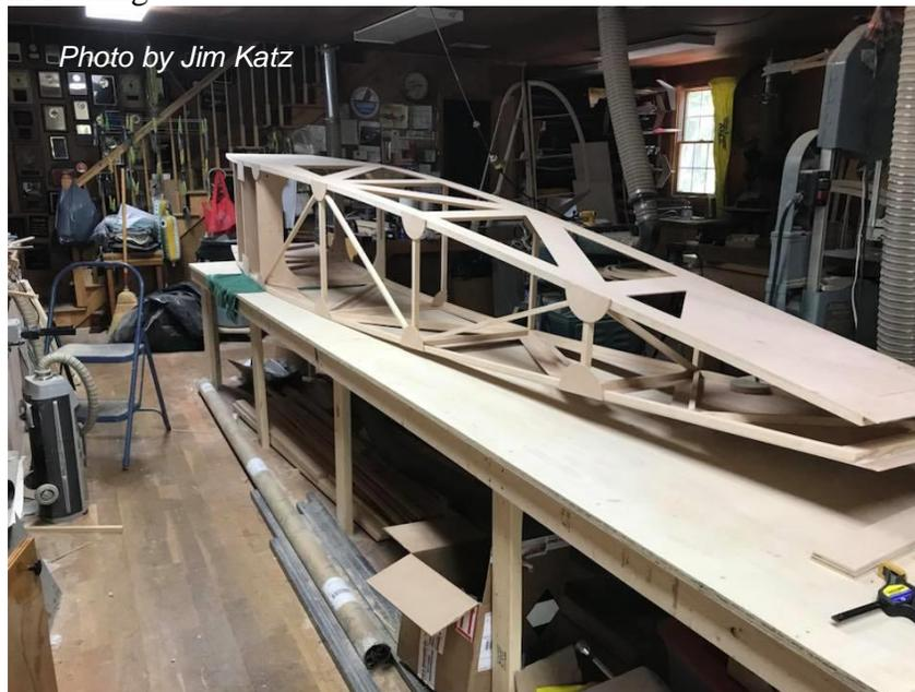
Figure 6: Laying the Fuselage on Its Side
