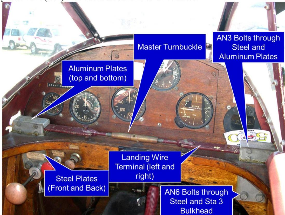
Figure 19: Landing Wire Support Assemblies
