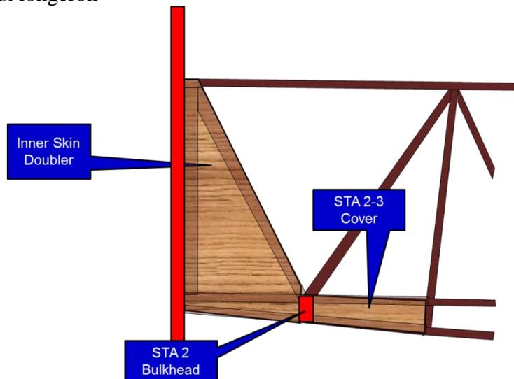
*Figure 12: Forward Inner Reinforcement*
