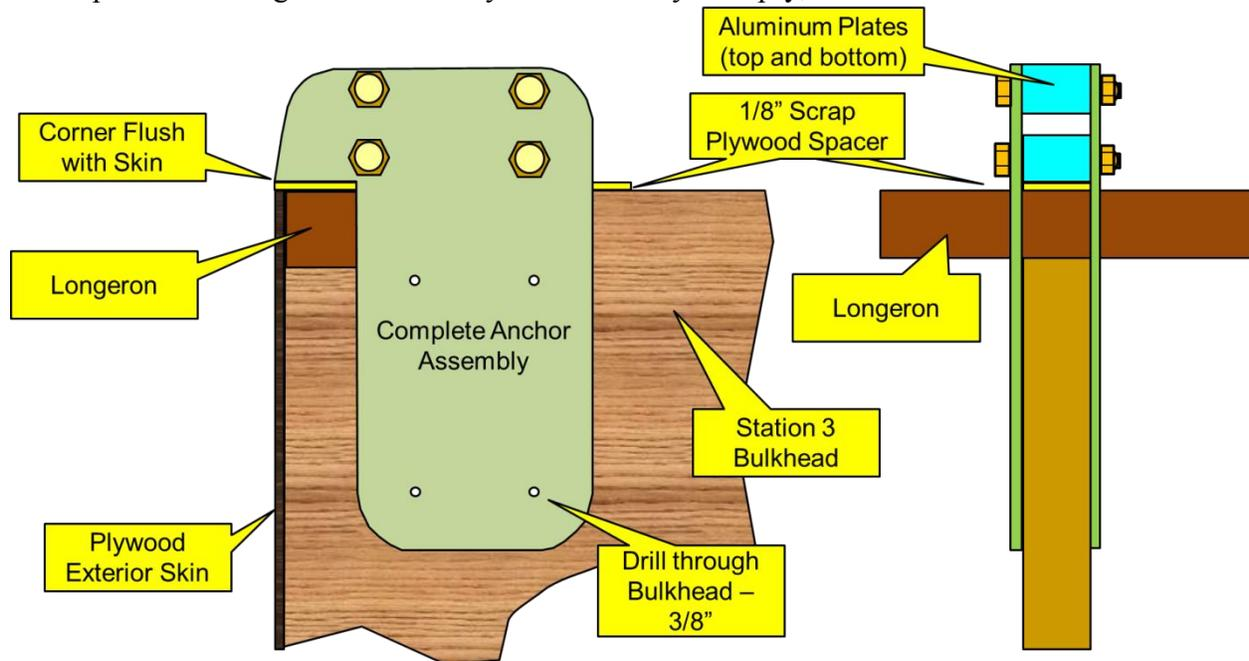
Figure 20: Landing Wire Anchor Installation
