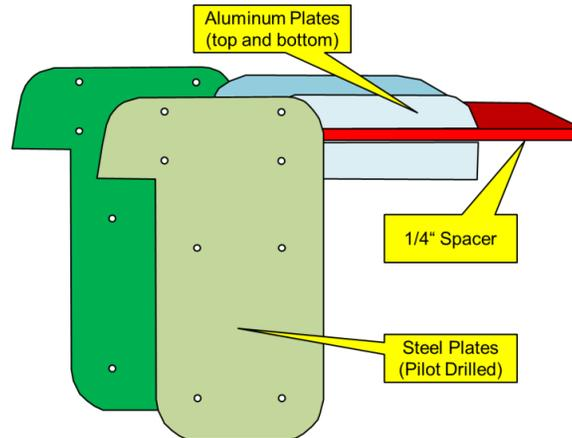
Figure 18: Landing Wire Anchors
