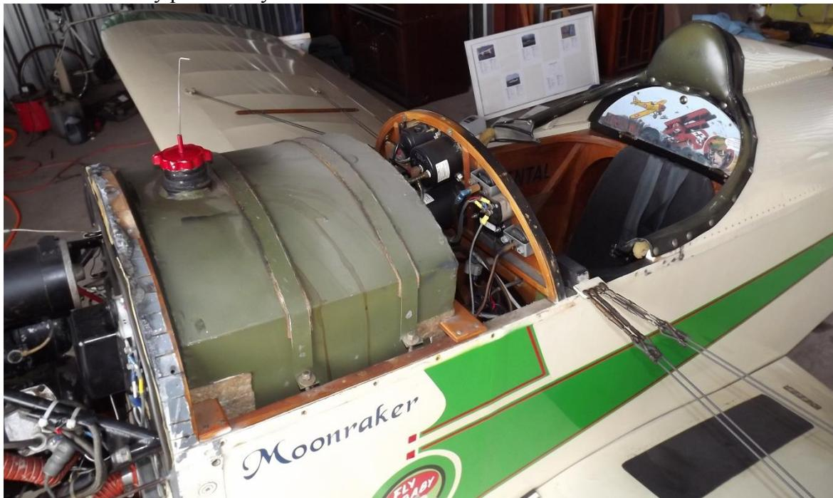
Figure 30: Fly Baby With Forward Turtledeck Cover Removed
