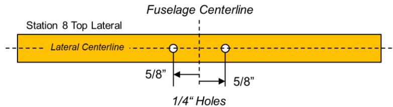
Figure 32: Holes in Station 8 Top Lateral
