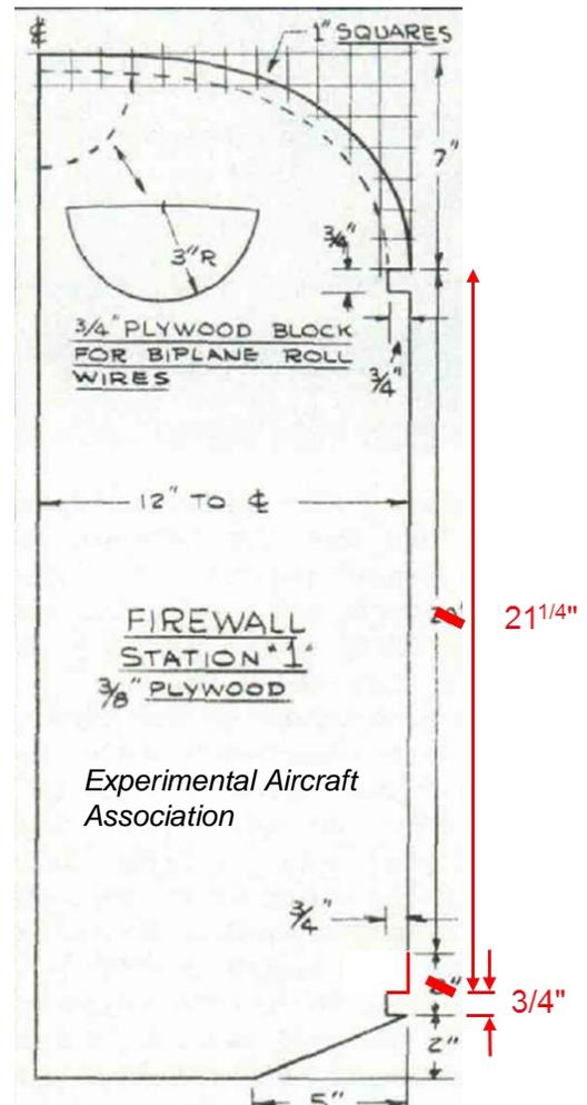
Figure 4: Corrected Firewall
