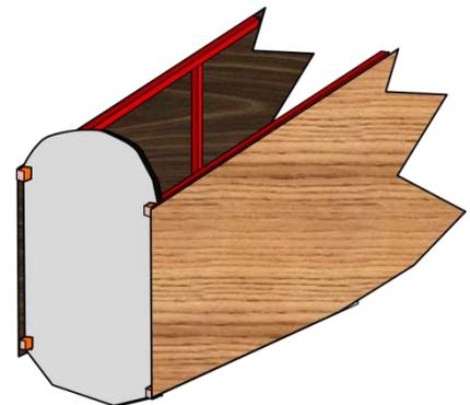
*Figure 8: Firewall with Plywood covering*
