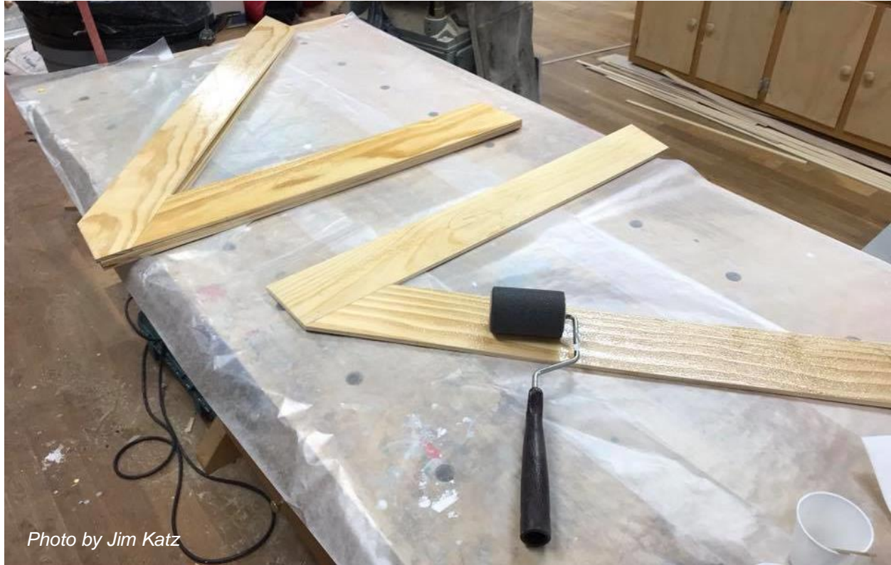
Figure 14: Using a Foam Roller to Apply Glue to Gear Laminations
