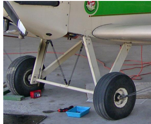
Figure 54: Gear Brace Wires
