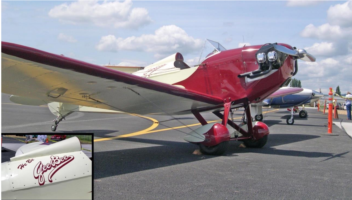
Figure 74: Installed Wheel Pants
