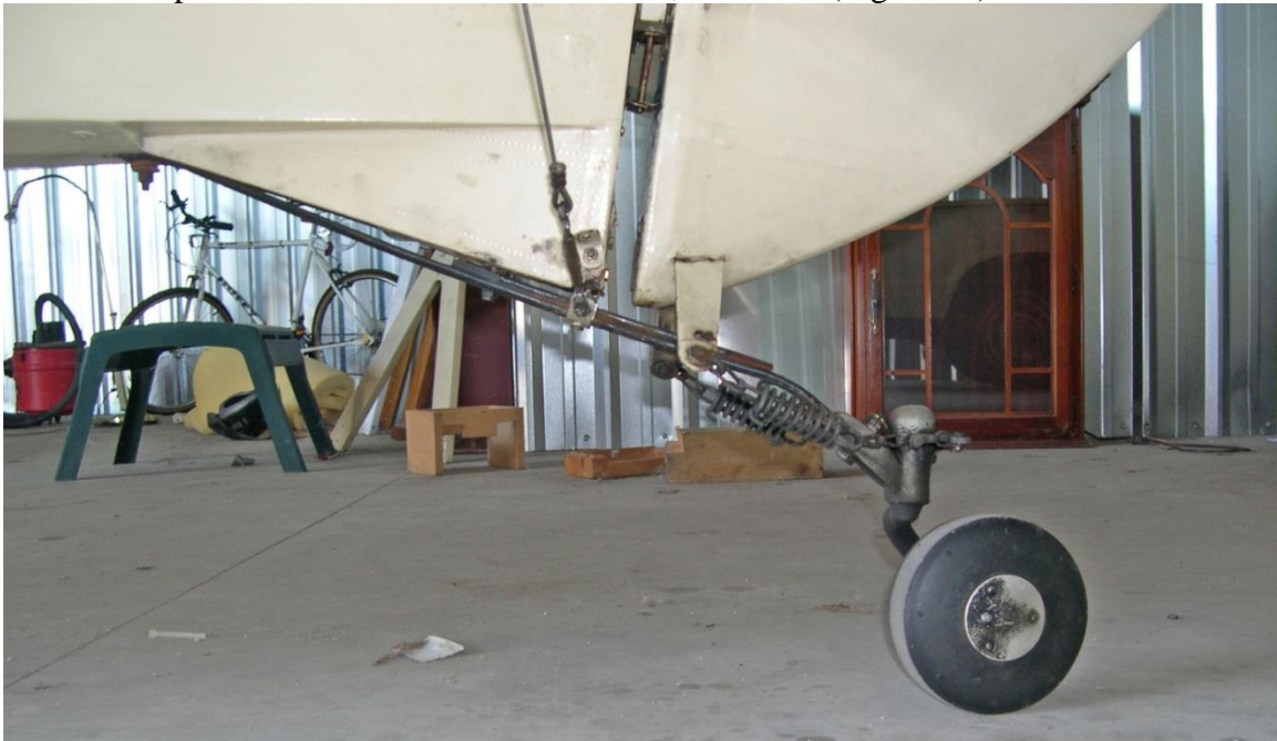
Figure 63: Ron's Tailwheel Installation
