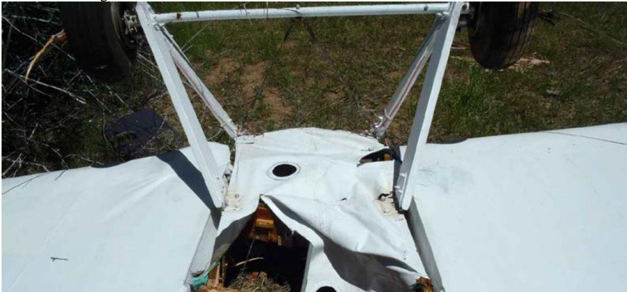
Figure 7: Intact Landing Gear Post-Crash
