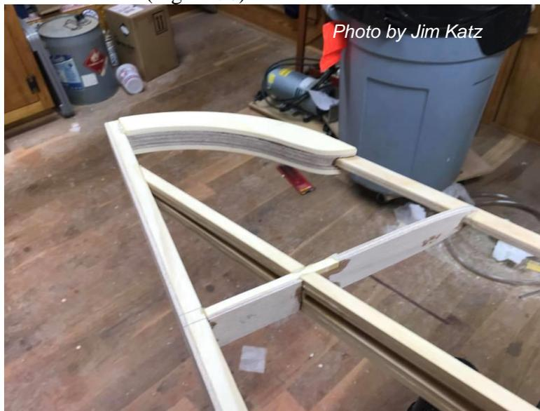
Figure 30: Horizontal Stabilizer Tip (Pre-Carving)
