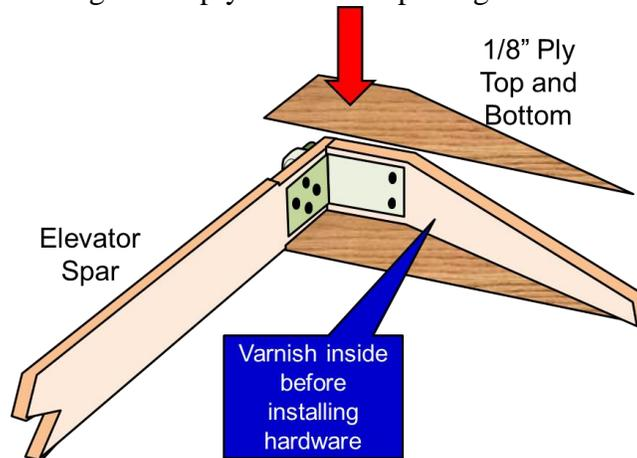
Figure 51: Elevator Root Plywood
