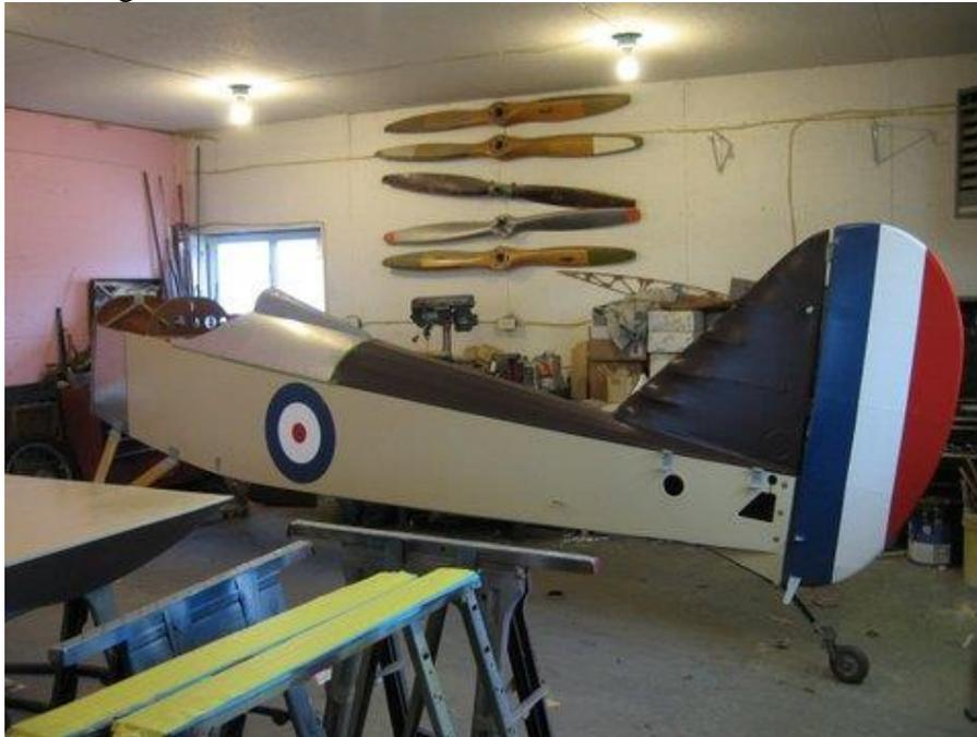
*Figure 65: Modified Rudder Shape – Curved*
