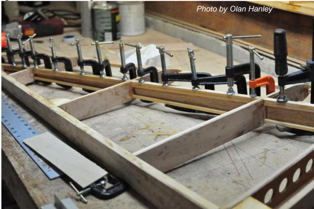
*Figure 31: Installing Filler Strips atop the Diagonal Spar*
