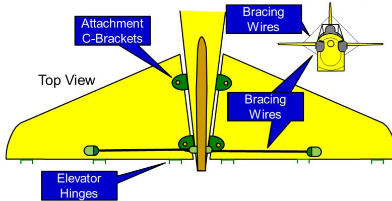
Figure 53: Horizontal Stabilizer Installation
