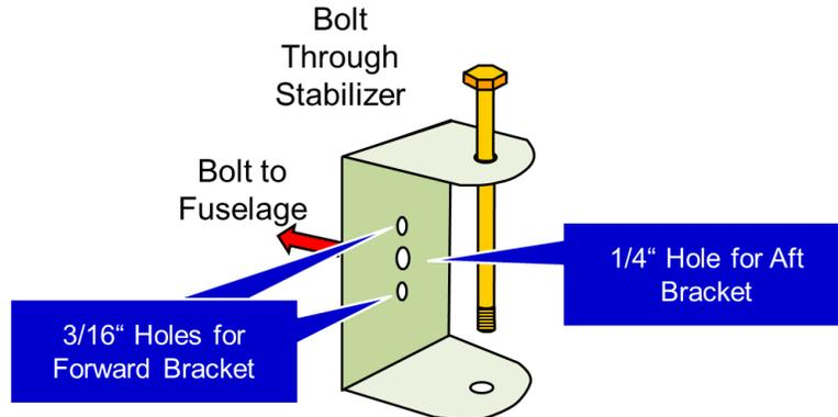
Figure 42: Horizontal Stabilizer Attachment Brackets
