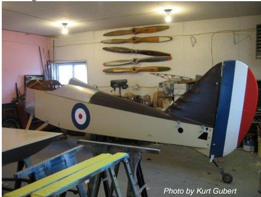
*Figure 65: Modified Rudder Shape – Curved*
