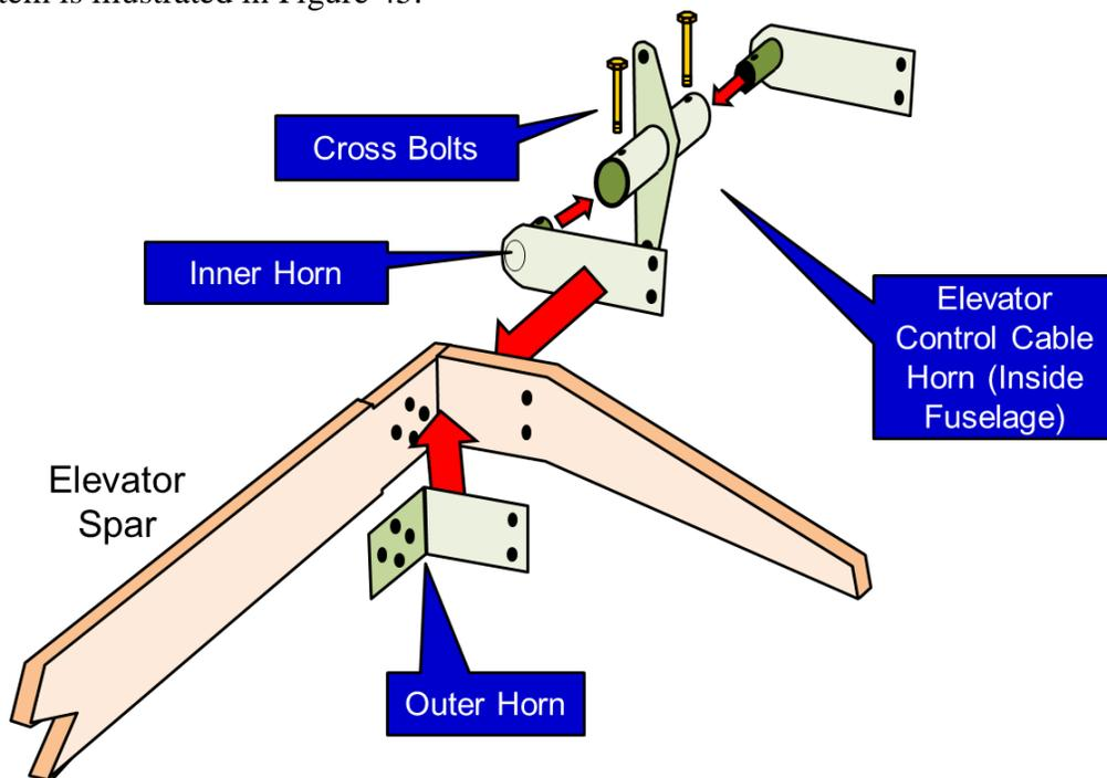
Figure 45: Elevator Control System
