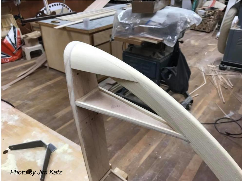
*Figure 22: Shaped Rudder Tip*
