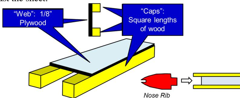
Figure 12: "Cap and Web" Rib Construction
