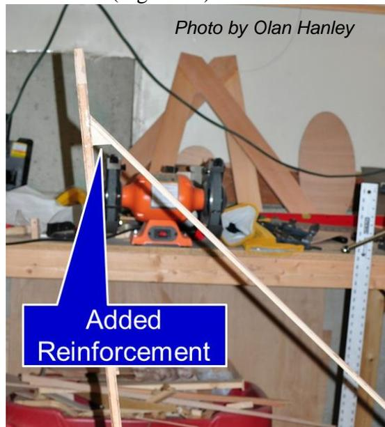
*Figure 15: Block Added to Top of Fin Diagonal Spar*
