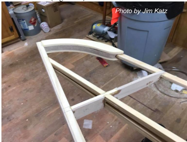
Figure 30: Horizontal Stabilizer Tip (Pre-Carving)
