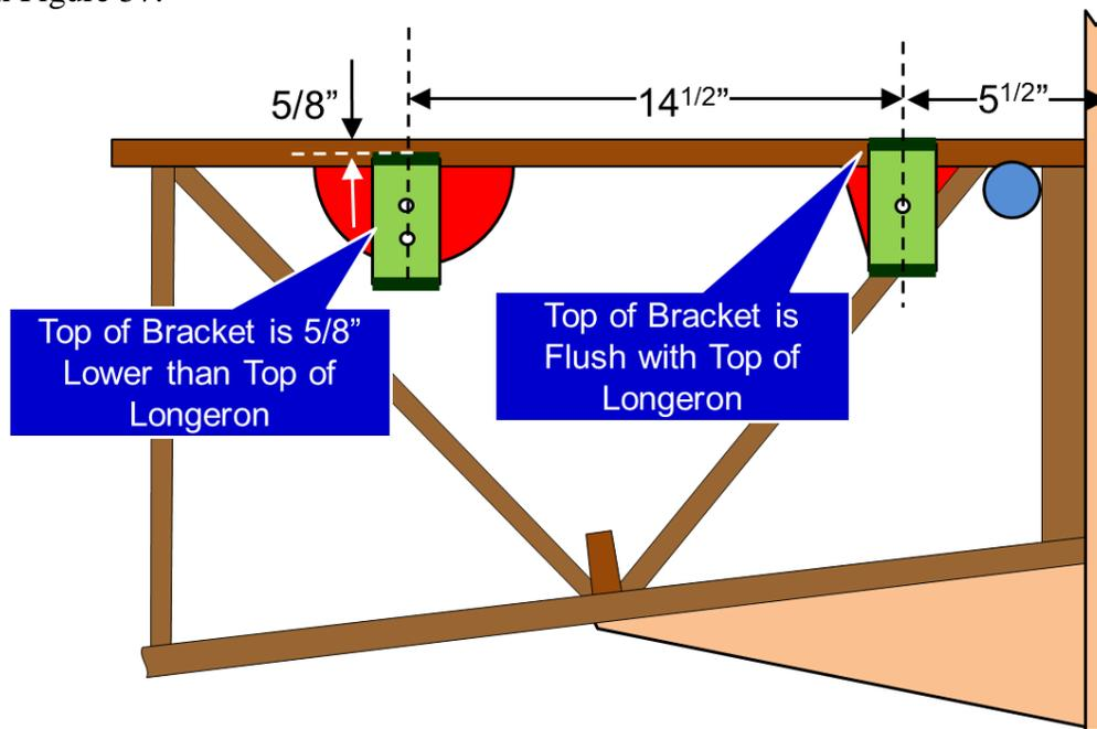
Figure 57: C-Bracket Positioning
