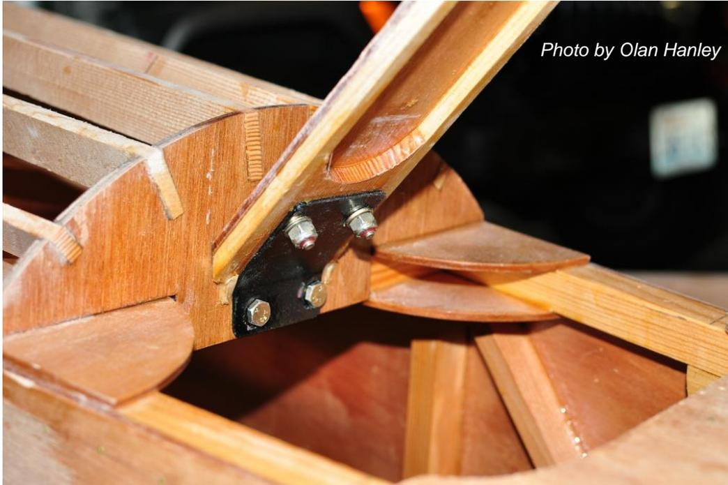
*Figure 14: Attaching the Bottom of the Fin Diagonal Spar*
