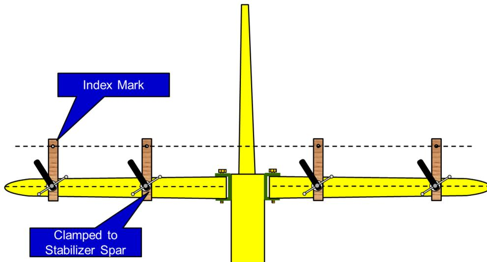
Figure 62: Horizontal Stabilizer Vertical Alignment
