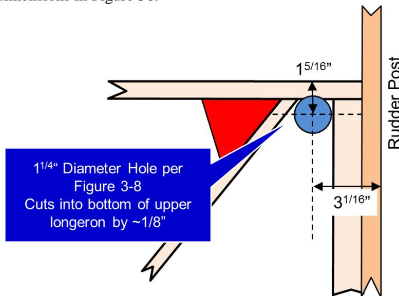
Figure 56: Control Horn Pass-Through Hole
