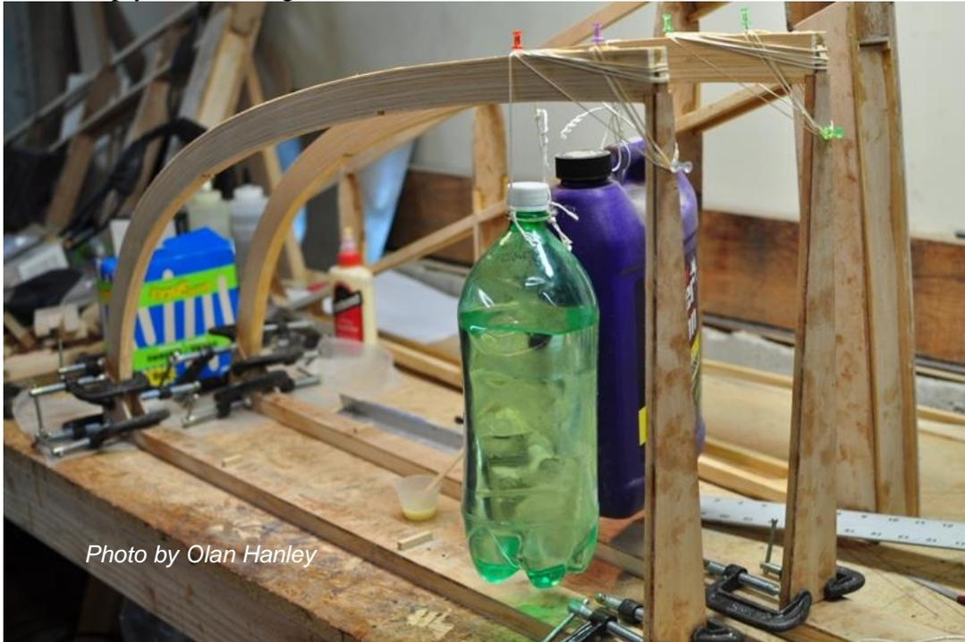
*Figure 37: Elevator Construction*
