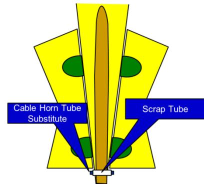
Figure 59: Using Scrap Tubes to Fit Elevators
