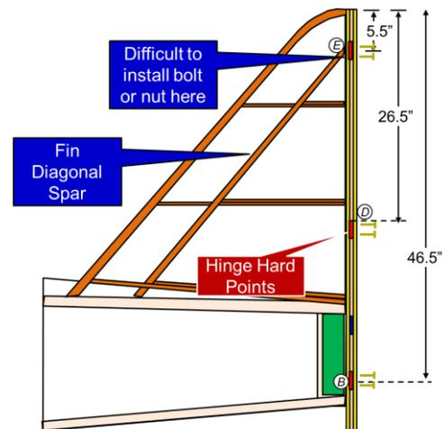
Figure 4: Interference Issue with Upper Hinge Point
