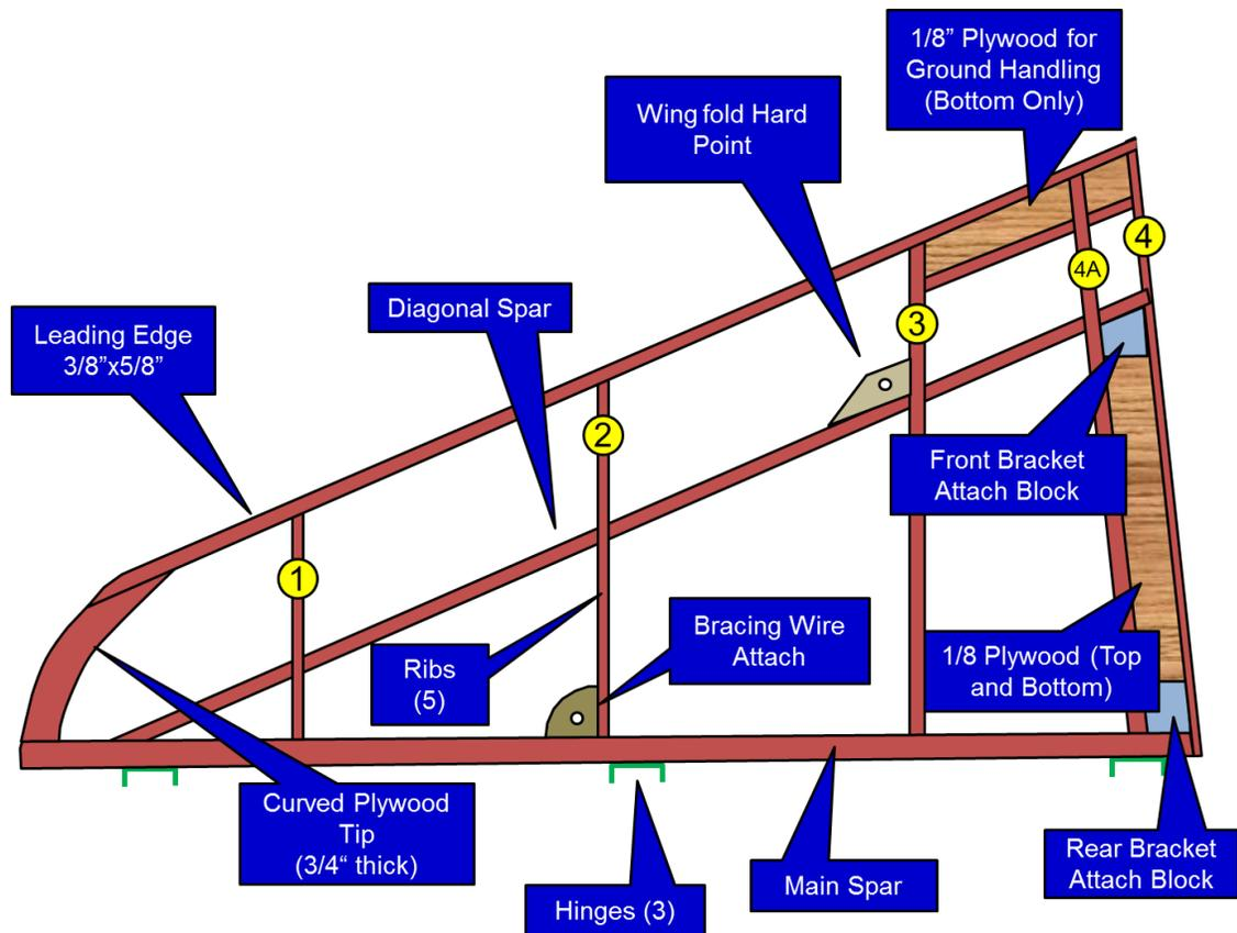
Figure 23: Horizontal Stabilizer Components
