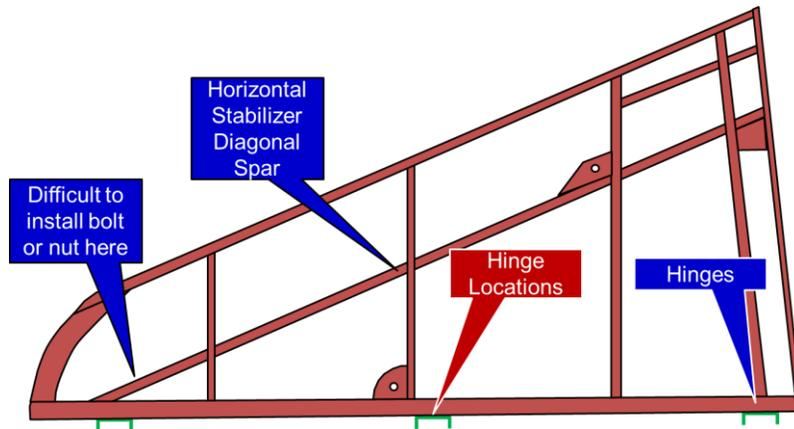
Figure 5: Horizontal Stabilizer Hinge Point Interference
