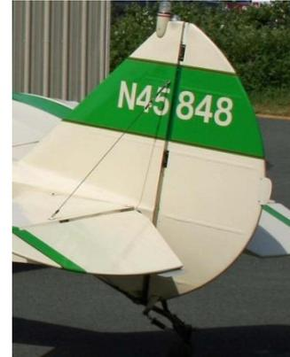
Figure 44: Tail Bracing
