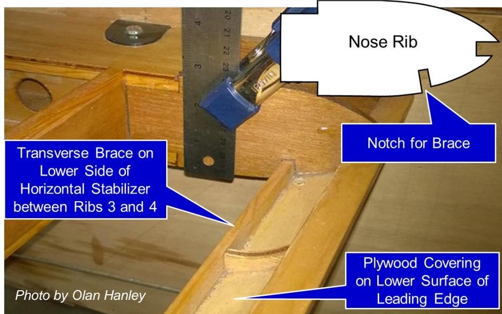
Figure 52: Horizontal Stabilizer Lift Support
