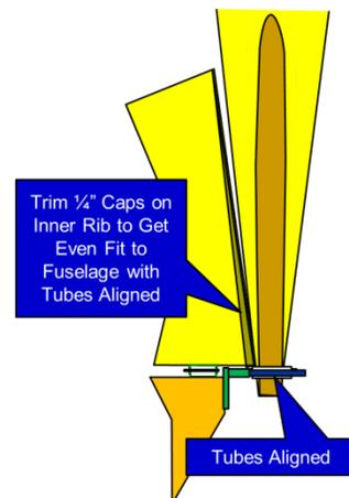
Figure 60: Trim Stabilizer to Match Fuselage
