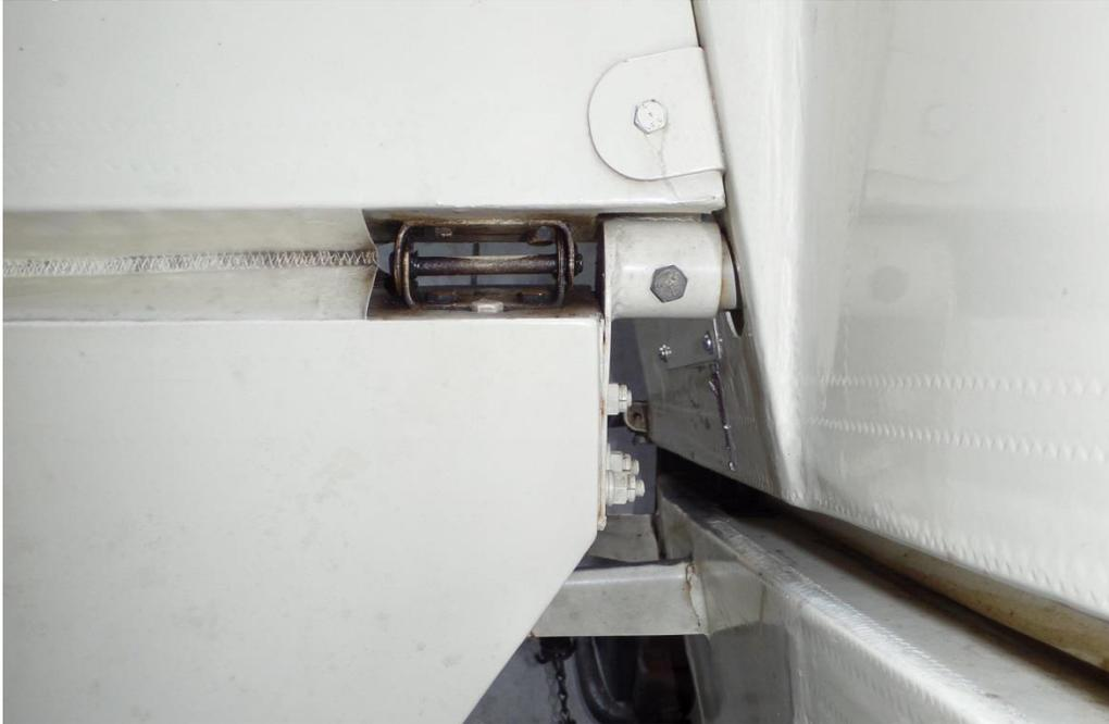
*Figure 46: Elevator Control Horn and Elevator Hinge*
