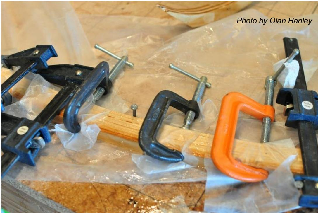
*Figure 34: Rudder Bow Construction*
