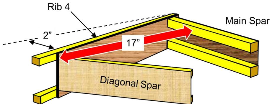
Figure 29: View of Rib 4/Diagonal Spar Interface
