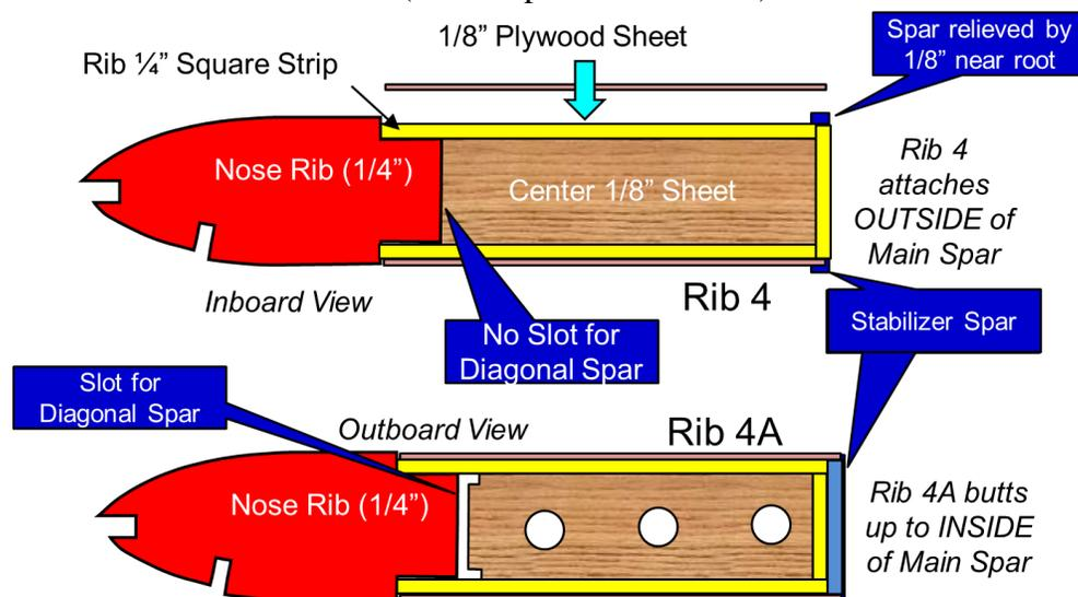
Figure 27: Horizontal Stabilizer Ribs 4 and 4A
