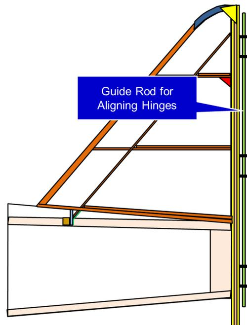
Figure 38: Hinge Installation
