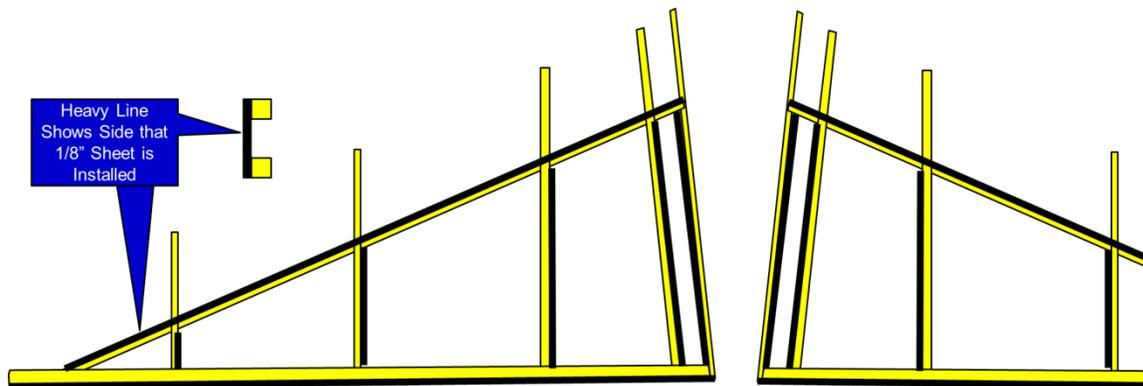
Figure 24: Face Sheet Orientation on Horizontal Stabilizers
