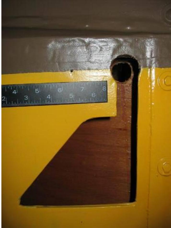
Figure 67: Modified Inspection Hole, can be added after completion and adjusted based on personal preferences. If a left-turning engine is eventually installed, the tab can just be bent the other way.
