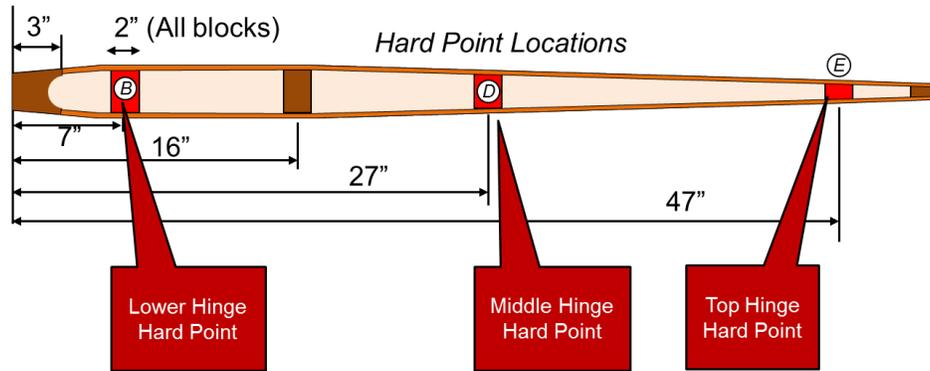
Figure 3: Rudder Post Dimensions
