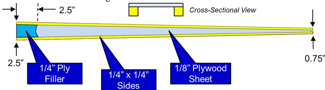
Figure 13: Fin Diagonal Spar
