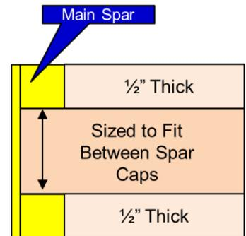
*Figure 32: Wire Anchor Block Cross-Section*
