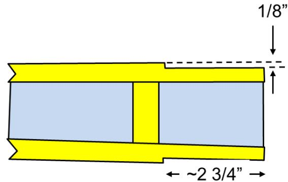
Figure 25: Detail of Spar Root
