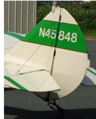
Figure 44: Tail Bracing
