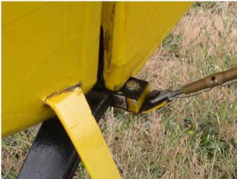
*Figure 64: Bracing Wires Attached to Tailwheel Spring Clamp*
