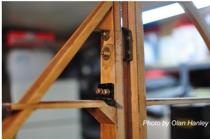
Figure 43: Fin Brace Wire Attach Fitting
