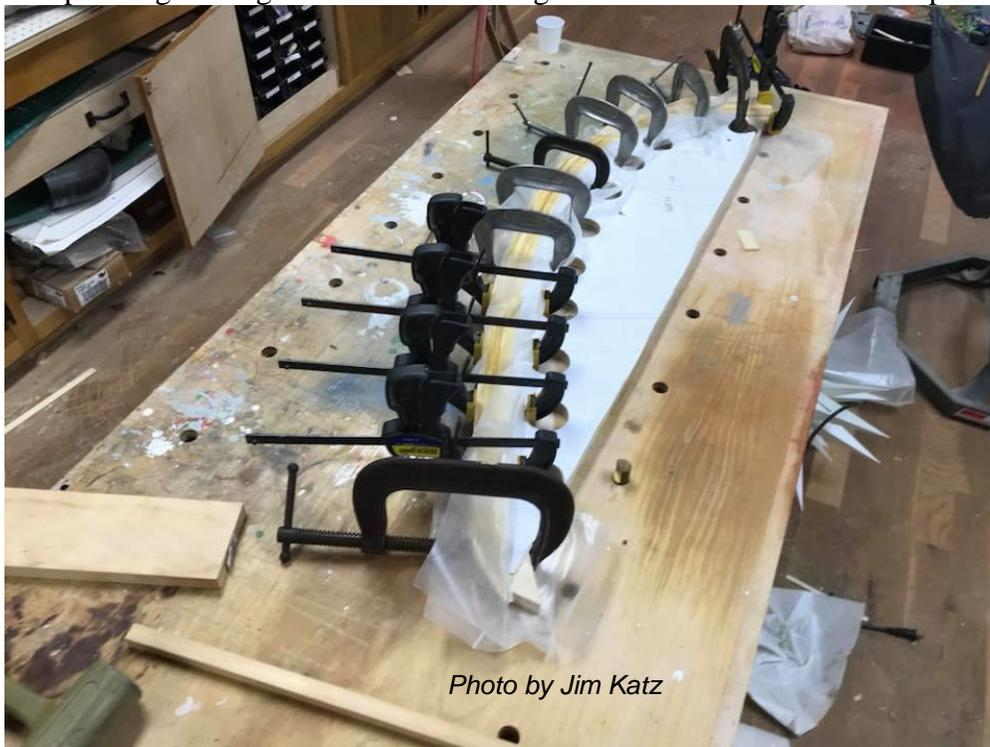
*Figure 35: Form used for Alternate Lamination Process*
