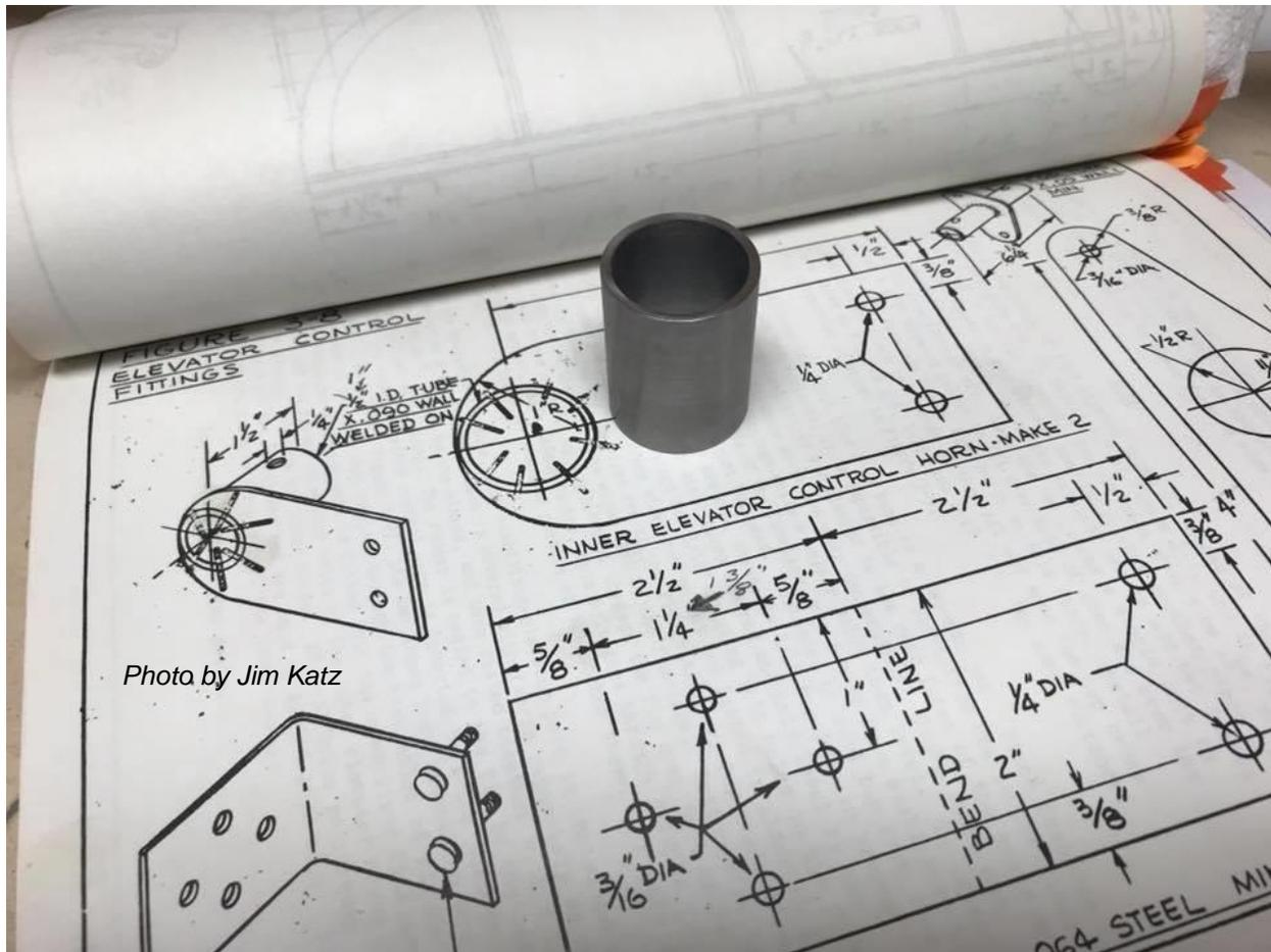
Figure 8: Elevator Horn Tube
