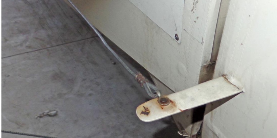
Figure 8: Slack in Rudder Cable
