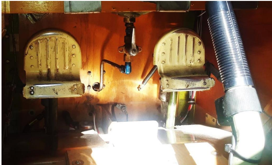
Figure 52: Rudder Pedals with Toe Brakes
