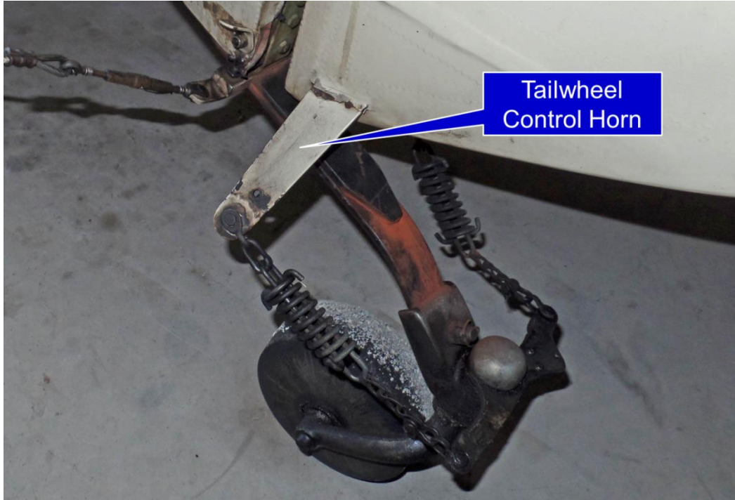
Figure 54: Bend in Tailwheel Control Horn
