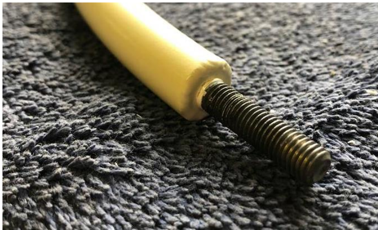
Figure 14: Threaded Rod End Made From Grade 5 Bolt
