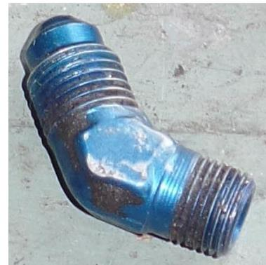
Figure 20: AN Flare and Pipe Thread
