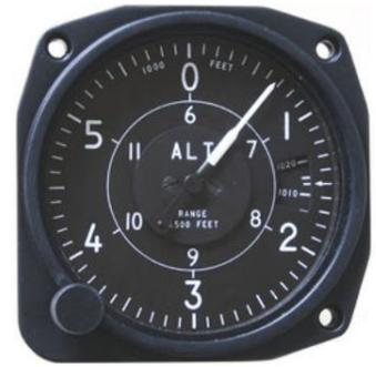
*Figure 26: Non-Sensitive Altimeter*
