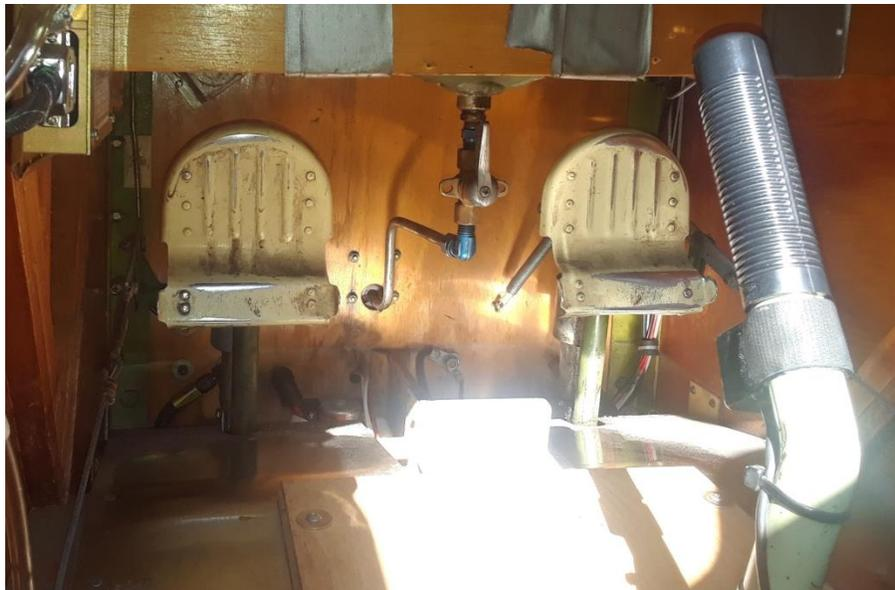
*Figure 12: Cessna 140 Rudder Pedals/Toe Brakes on a Fly Baby*
