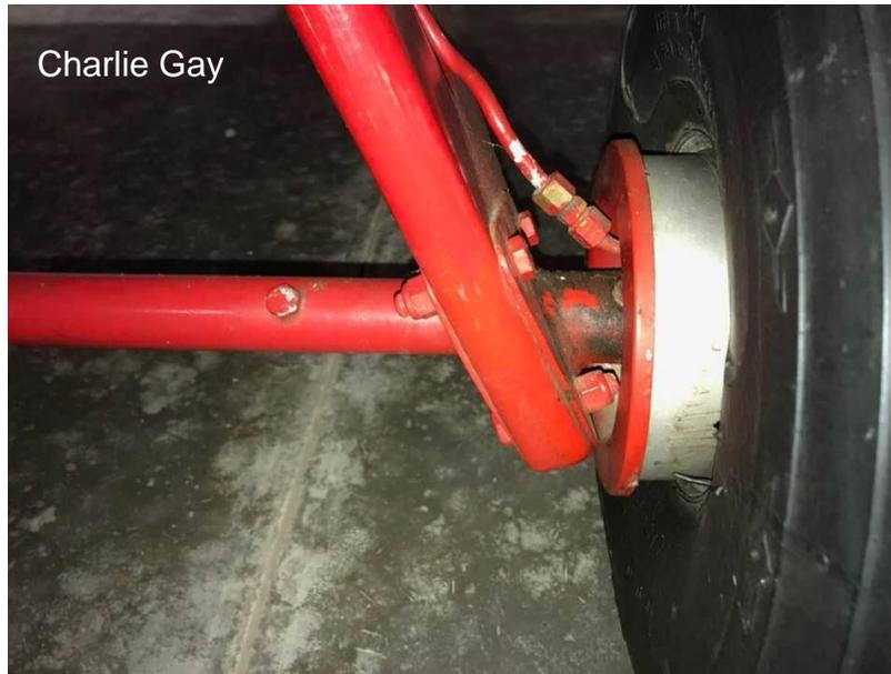
*Figure 9: Drum Brakes*
