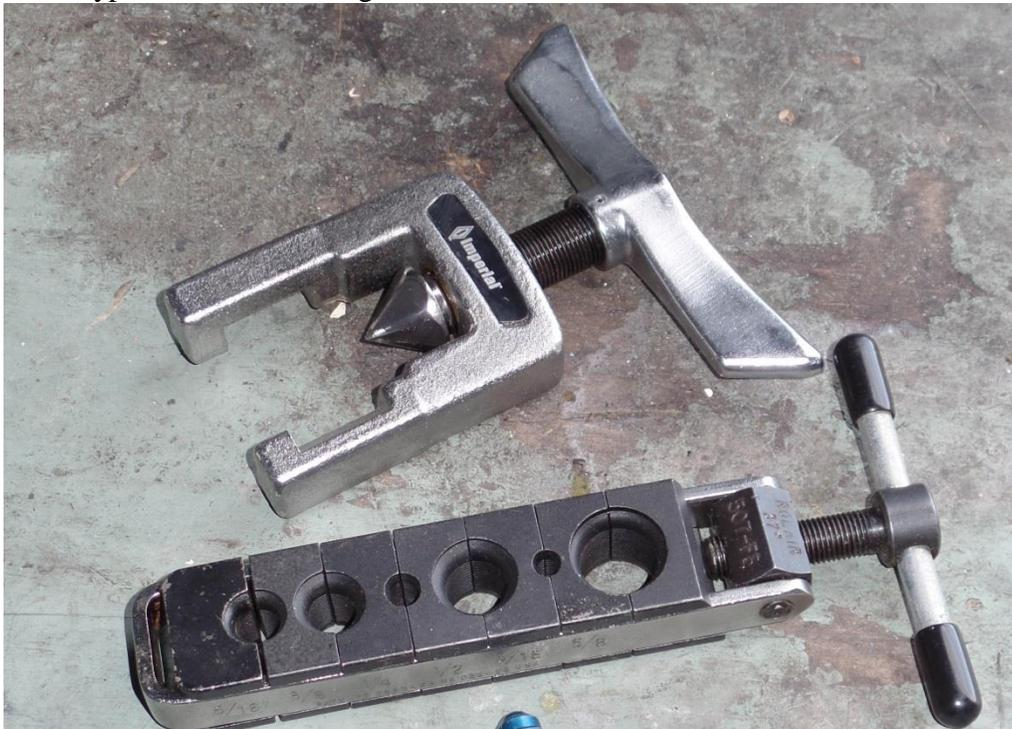
*Figure 18: Tubing Flare Tool*
