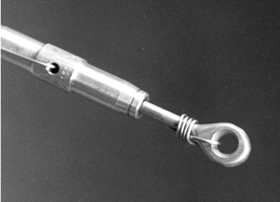
The single-wrap method can be used on turnbuckles connected to 1/8-inch or smaller cables. Brass safety wire is acceptable on 1/16-inch and 3/32-inch cables, but stainless steel is required for 1/8 inch. Whichever type is used, it must be at least 0.040 inch in diameter. Cables 5/32 inch and larger can be single-wrapped, but only with .057-inch stainless steel. This thicker wire is harder to bend.
