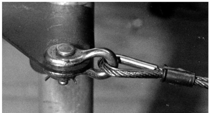
shackle indicates its rated strength in hundreds of pounds. An AN115-21 shackle, for instance, is rated at 2,100 pounds. This is the smallest shackle that can be used with 3/32-inch or 1/8-inch cable.
