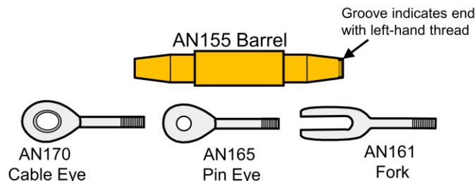
A barrel is combined with two ends to form standard assemblies:
