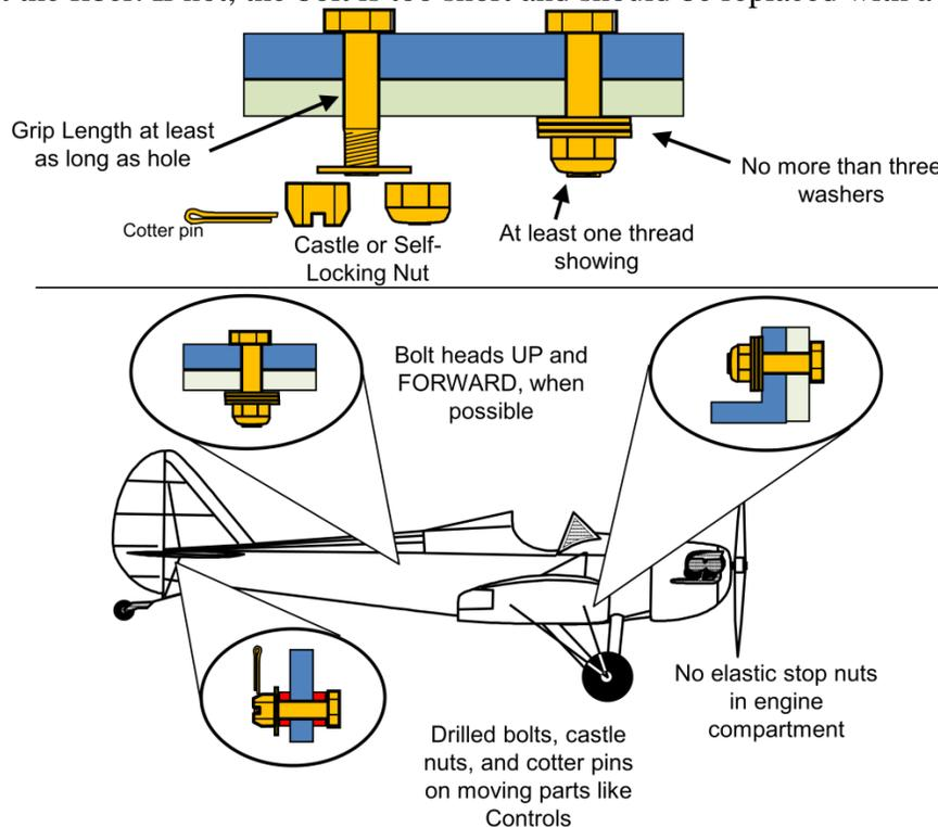
If there are more than three threads showing, the bolt might be too long. Try to rotate the bolt with the wrench without holding the other end. If it turns, the nut bottomed out before proper pressure could be applied. Remove the nut and add another washer. Re-tighten, recheck,
