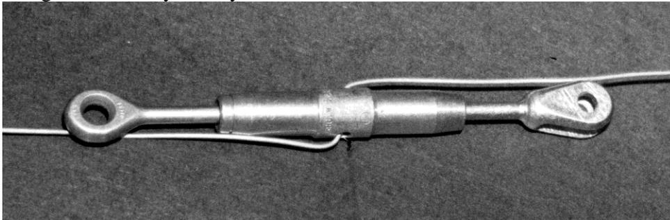
Wrap the ends of the wire around the shanks of the turnbuckle ends at least four times and cut off the excess.
