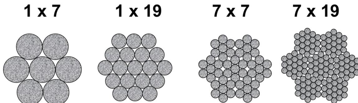
Single-strand cable is best for bracing and other applications that don't pass through fairleads or pulleys, so you'll see 1x19 specified for Fly Baby wing bracing. The so-called flexible cables (7 x 7 or 7 x 19) are best for control systems. The 7 x 19 construction is
