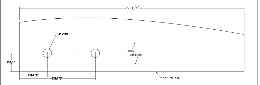
NOTE: I WOULD RECOMMED DRILLING  $\emptyset 3/4$  HOLES FIRST TO MAKE SURE EVERYTHING ALIGNS. THEN, GO BACK AND DRILL  $\emptyset 1.0$  HOLE AS PER PLANS, PAGE 4-17, STEP 10A.
