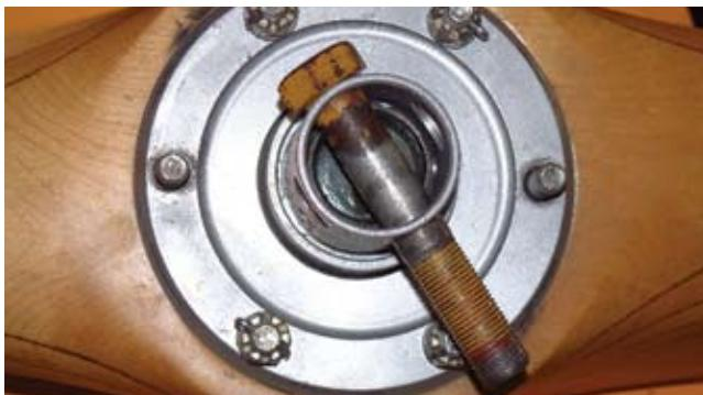
**A 5/8-inch by 4-inch Grade 8 bolt is inserted through the prop hub locking nut. Note that the spinner-mounting bracket has been removed for complete access to the hub.**
