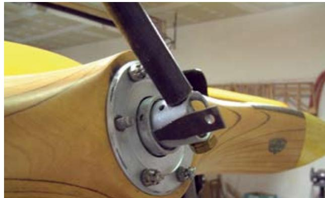
**The snap ring retention tool has been inserted into the snap ring opening, and the pipe extension is in place. The prop hub nut is now ready to be rotated counterclockwise approximately two to two-and-a-half turns.**
