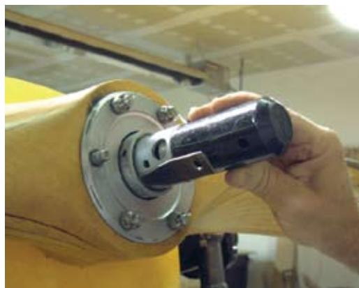
**This photo clearly shows the snap ring tool in place and the steel rod inserted into the locking hub nut. Note how the outer diameter of the steel rod rests firmly against the outer flat surface of the hub nut.**
