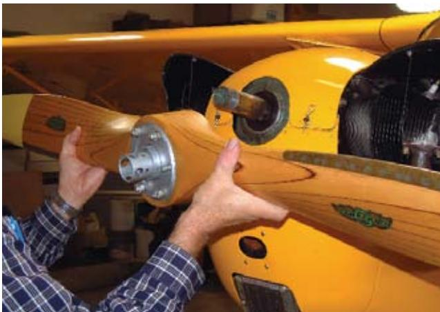
**Once the hub has popped free and the hub nut turned counterclockwise until free of the crankshaft threads, the prop can be guided off the shaft.**
