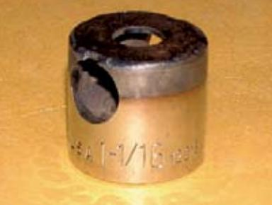
**We use another homemade tool for correctly torquing the prop hub nut, as it does require 200 to 225 foot-pounds of torque for proper installation. This tool is made using a 1/2 inch drive 1-1/16-inch socket. A flat washer, used for rigidity, is welded over the open socket end. Then a 5/8-inch diameter hole is drilled completely through the socket.**
