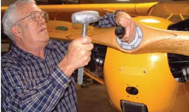
**While applying light pressure to the back side of the prop, insert the steel shaft into the hub nut and tap lightly with either a rubber mallet or lead hammer. The light pressure prevents the crankshaft journals from banging against the engine case when applying the light tapping to the inserted steel shaft.**
