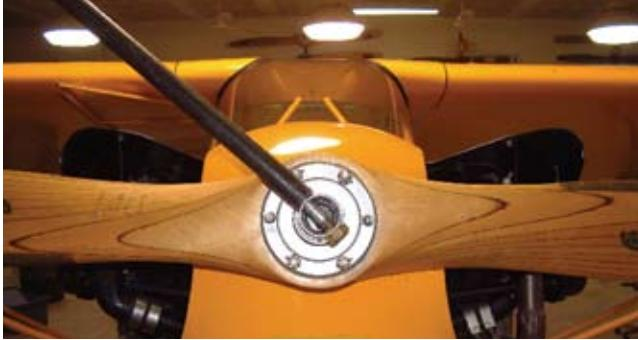
**The Grade 8 bolt has been inserted from the lower right to the upper left position in the hub nut, and a 30-inch length of 3/4-inch pipe has been slipped over the extended portion of the bolt. This position is used for ease in applying downward pressure on the pipe to loosen the hub nut.**
