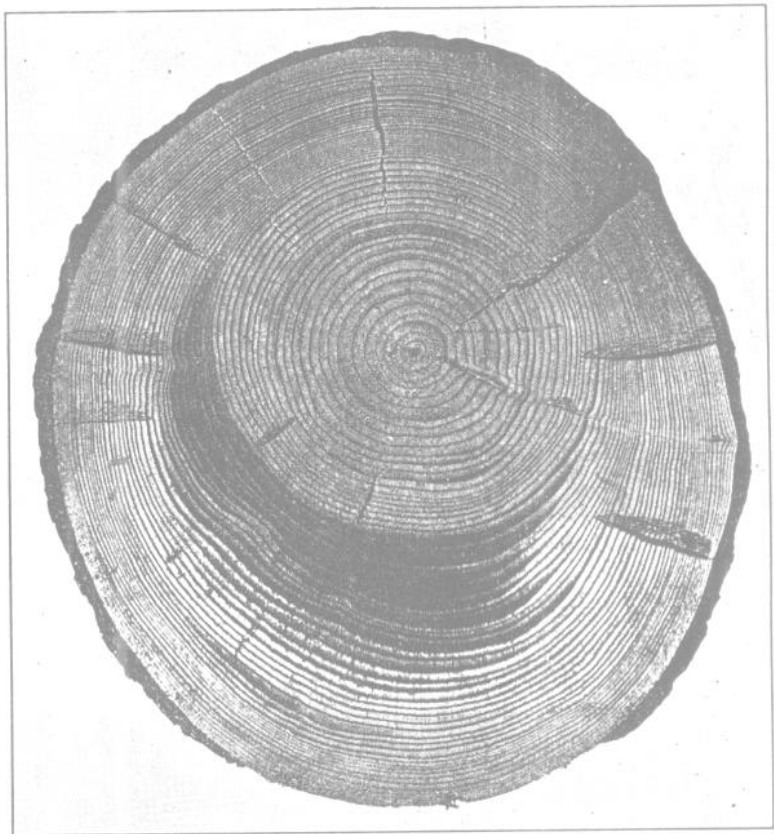
FIGURE 16.—Compression wood appearing as dark, wide portions of growth rings, in a cross section of an eastern spruce log
