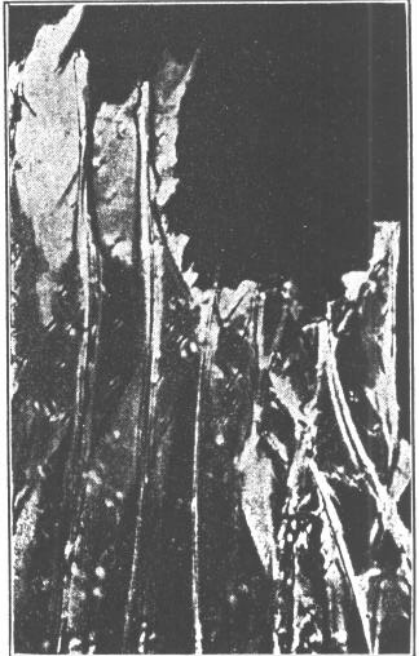
FIGURE 13.—Thin longitudinal section at a tension failure in spongy white ash, showing the spiral fracture of individual fibers and the corresponding slope of the slitlike pits in the fiber walls. The photograph was taken by polarized light. \times 350
