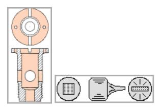
In order to use the torque wrench on the brass seat, a screwdriver with a wide and thick blade is needed to fit the segmented slot of the seat. This type of driver, made for a socket wrench, is the best solution.
