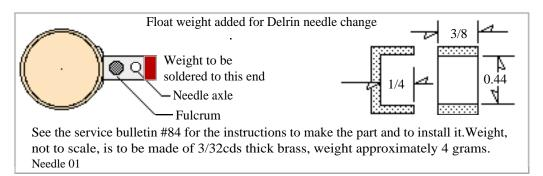
Recently, an Ercoupe owner had an engine failure during landing and ran into power lines near the end of the field; it was found that when the change was made to the Delrin needle and the weight required was added to the float, the weight or the solder to hold it on got hung up on the carburetor body, flooding the engine with full fuel flow, rendering the engine unable to develop power.
