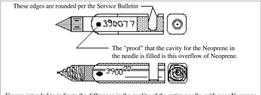
Figures intended to indicate the difference in the quality of the entire needle, with poor Neoprene surface finish and many machine marks indicative of poor shop practice.
