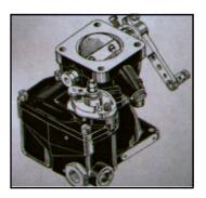
These carburetors were designed to use a stainless steel needle and sharpedged bronze seat. Not surprisingly, they would often leak and the only cure then was to lap them (see the article on "Needles" for how to do that
